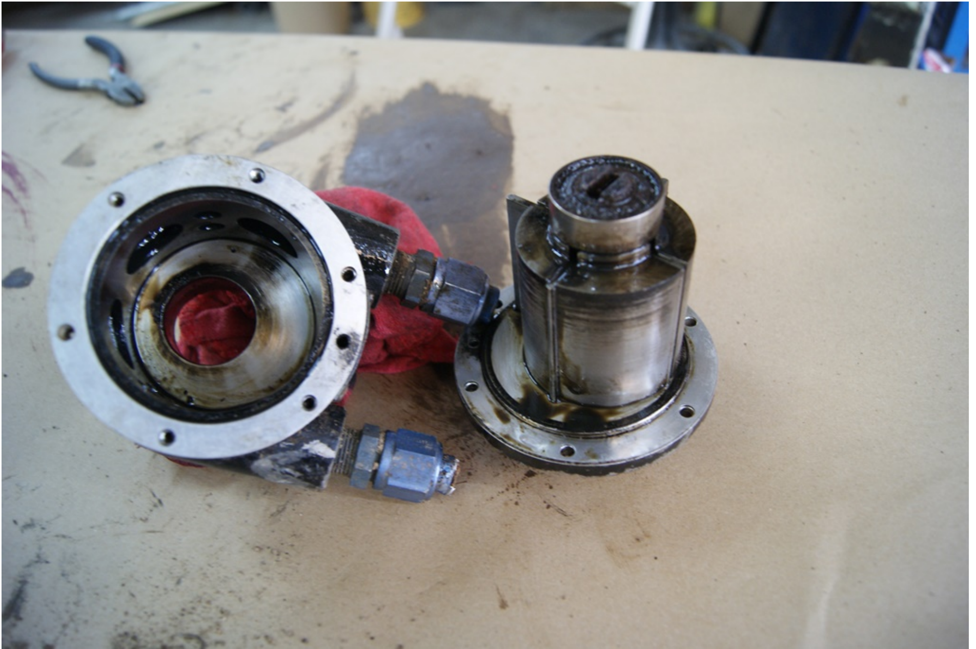
Photo 8 – Vacuum Pump Disassembly
