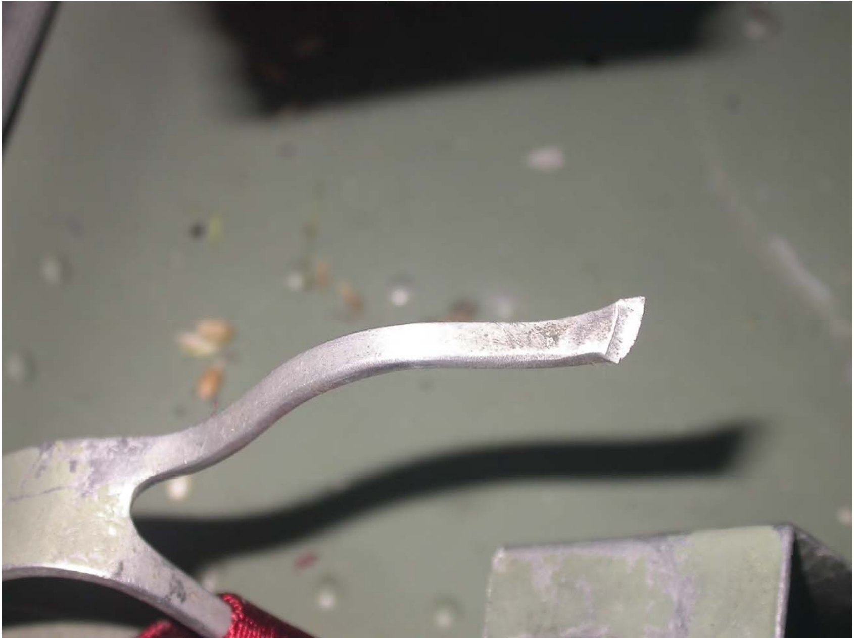
Photo 11 – Close Up of Broken Center Safety Belt Bracket
