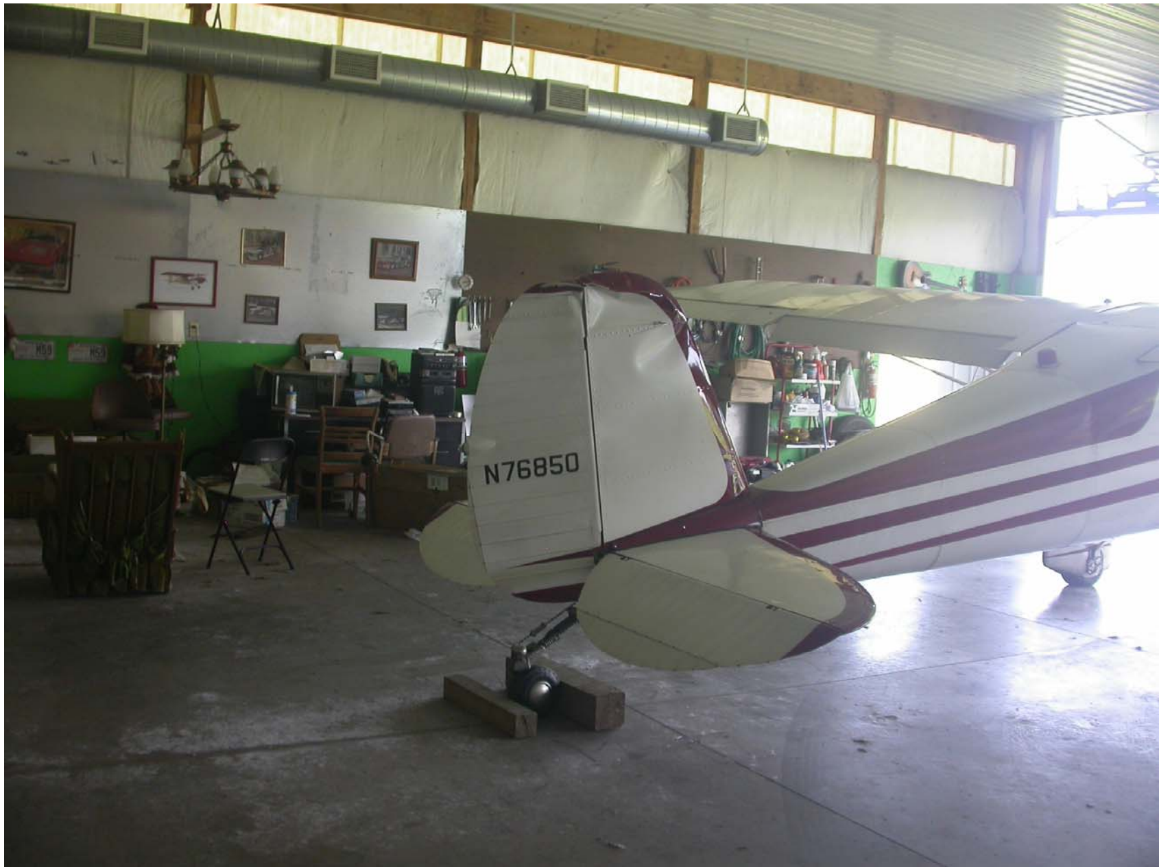
Photo 9 – Damage to Vertical Stabilizer and Rudder
