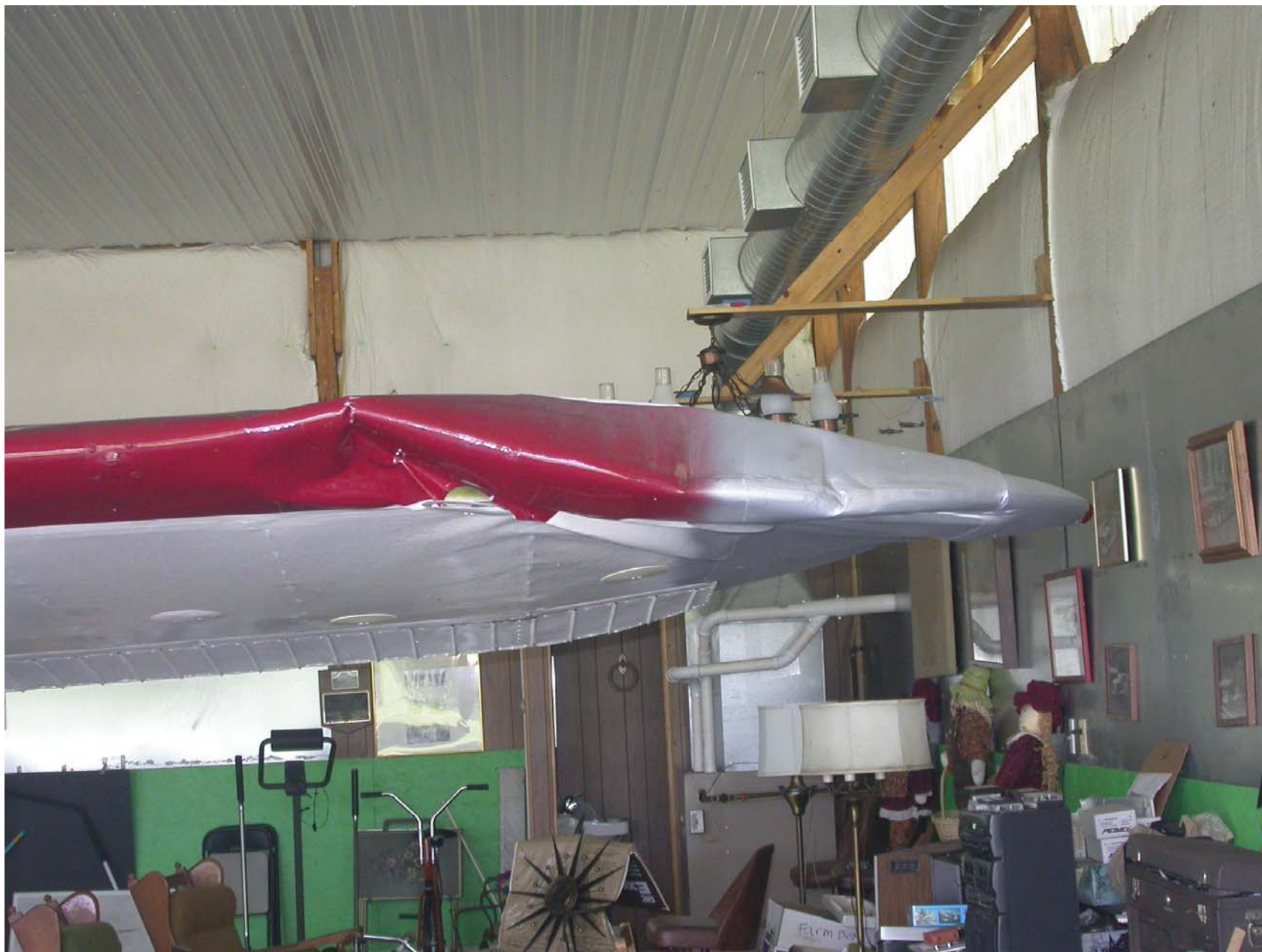
Photo 8 – Damage to Left Wing Tip
