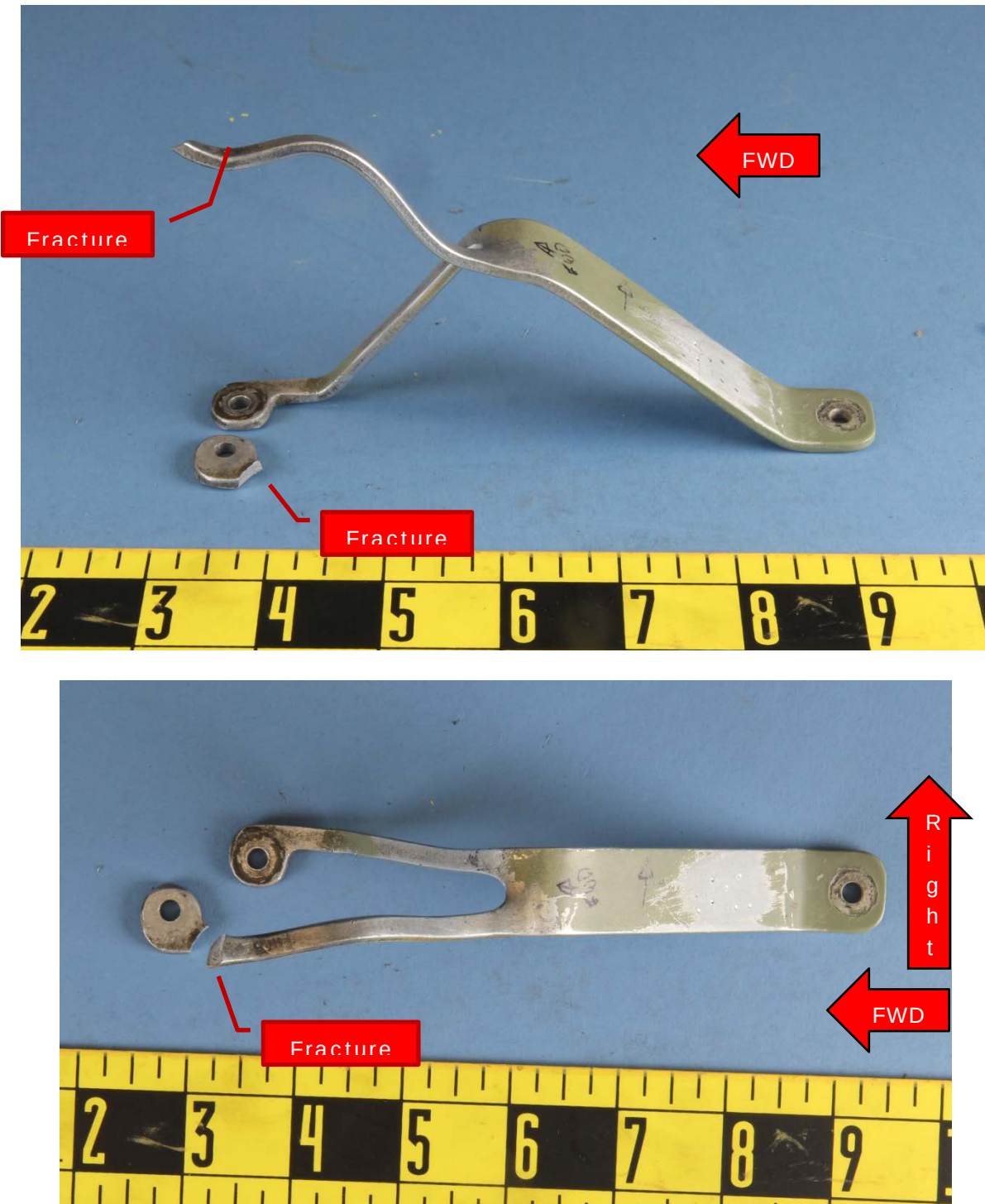
Figure 1. Two views of the fractured seat belt bracket, left side at top, top view below. The extent and shape of both the pre and post fracture deformation is visible in the side view at top.
