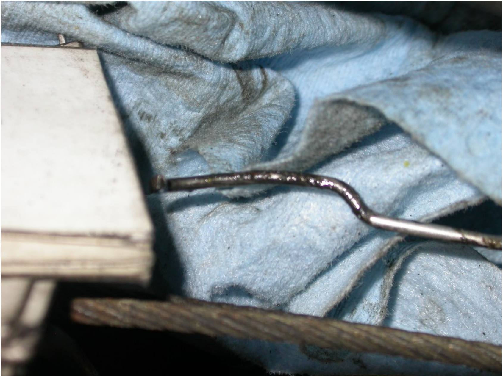
Photo 10 - Disconnected Right Fuel Valve Control Cable
