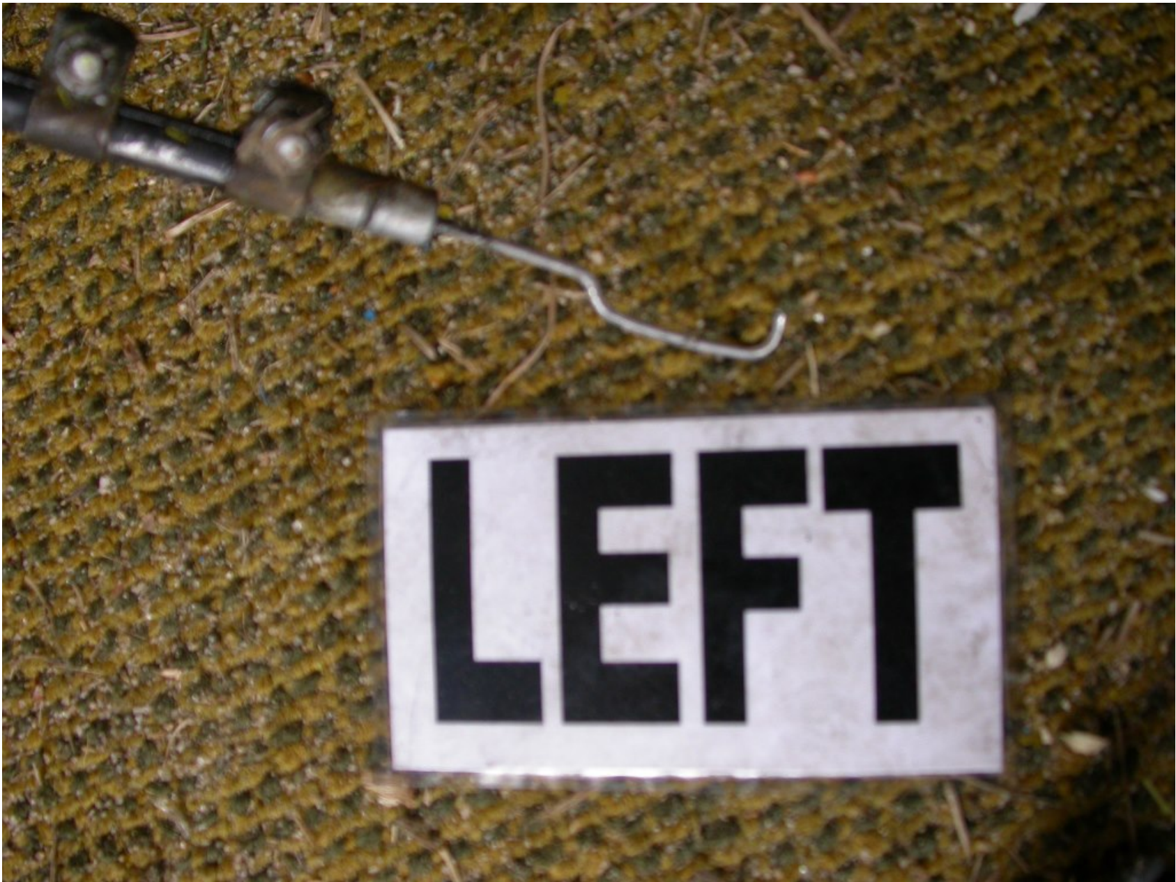
Photo 11 - Disconnected Left Fuel Valve Control Cable
