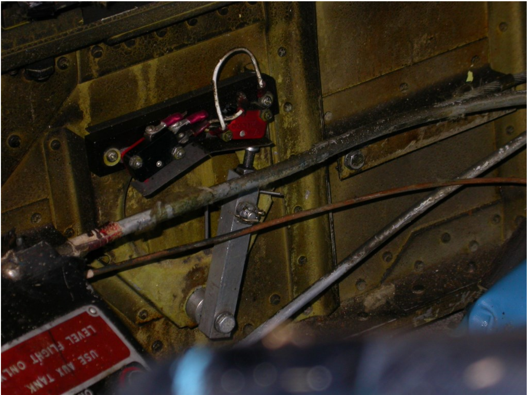
Photo 7 - Fuel Control Cable Support Arm as Found In Main Tank Position
