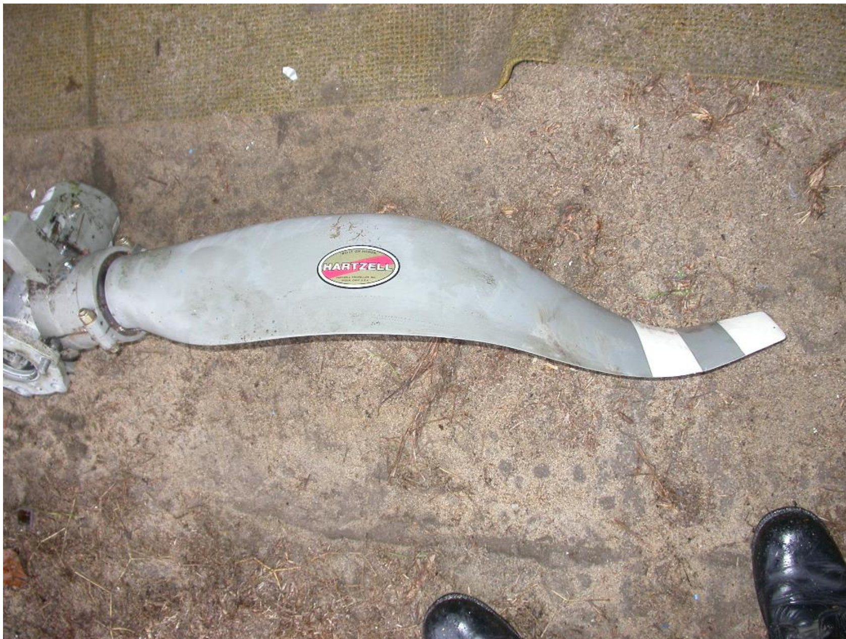
Photo 5 - Close Up of Bent Blade on Right Propeller
