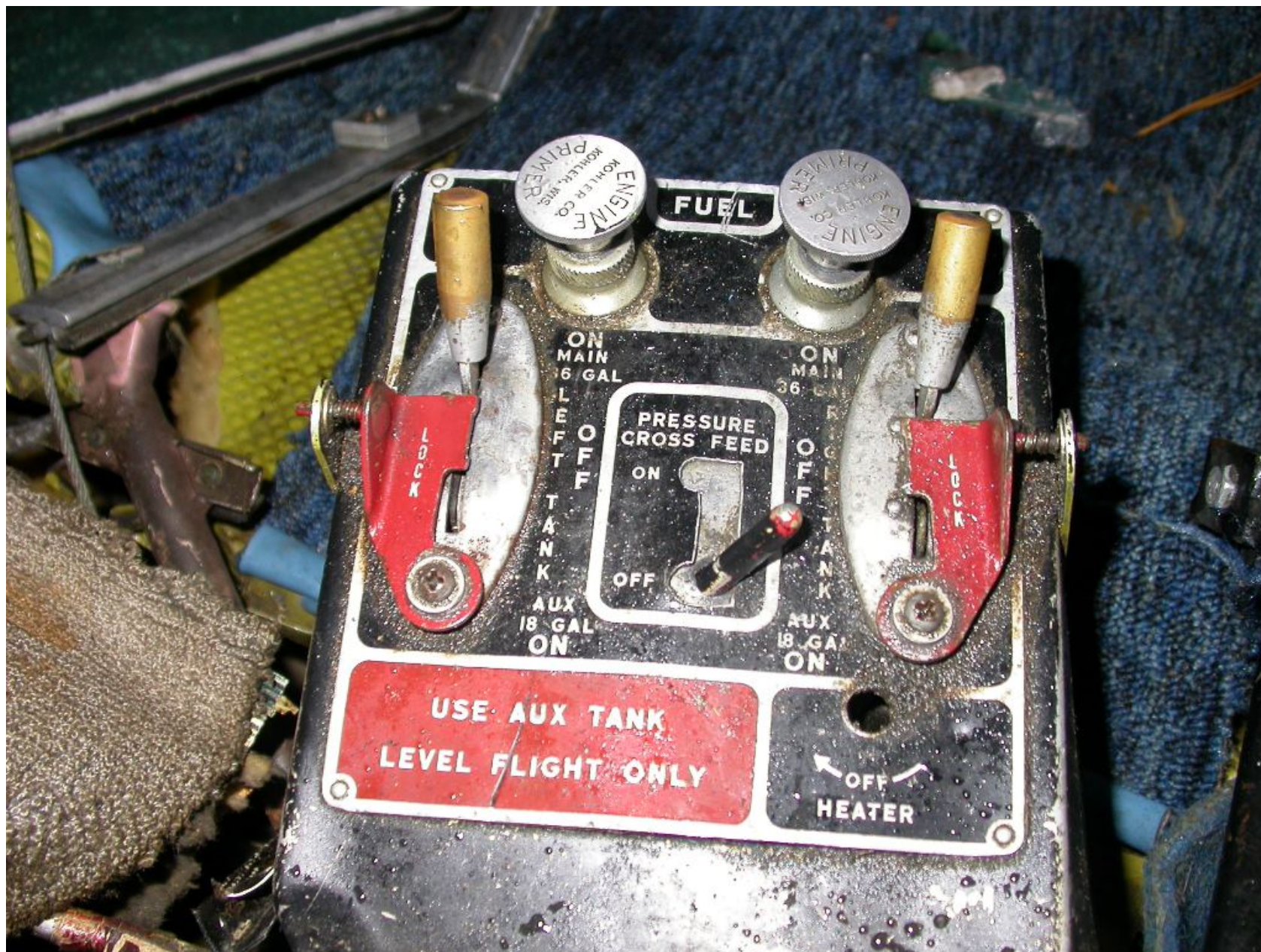
Photo 2 - Fuel Control Panel
