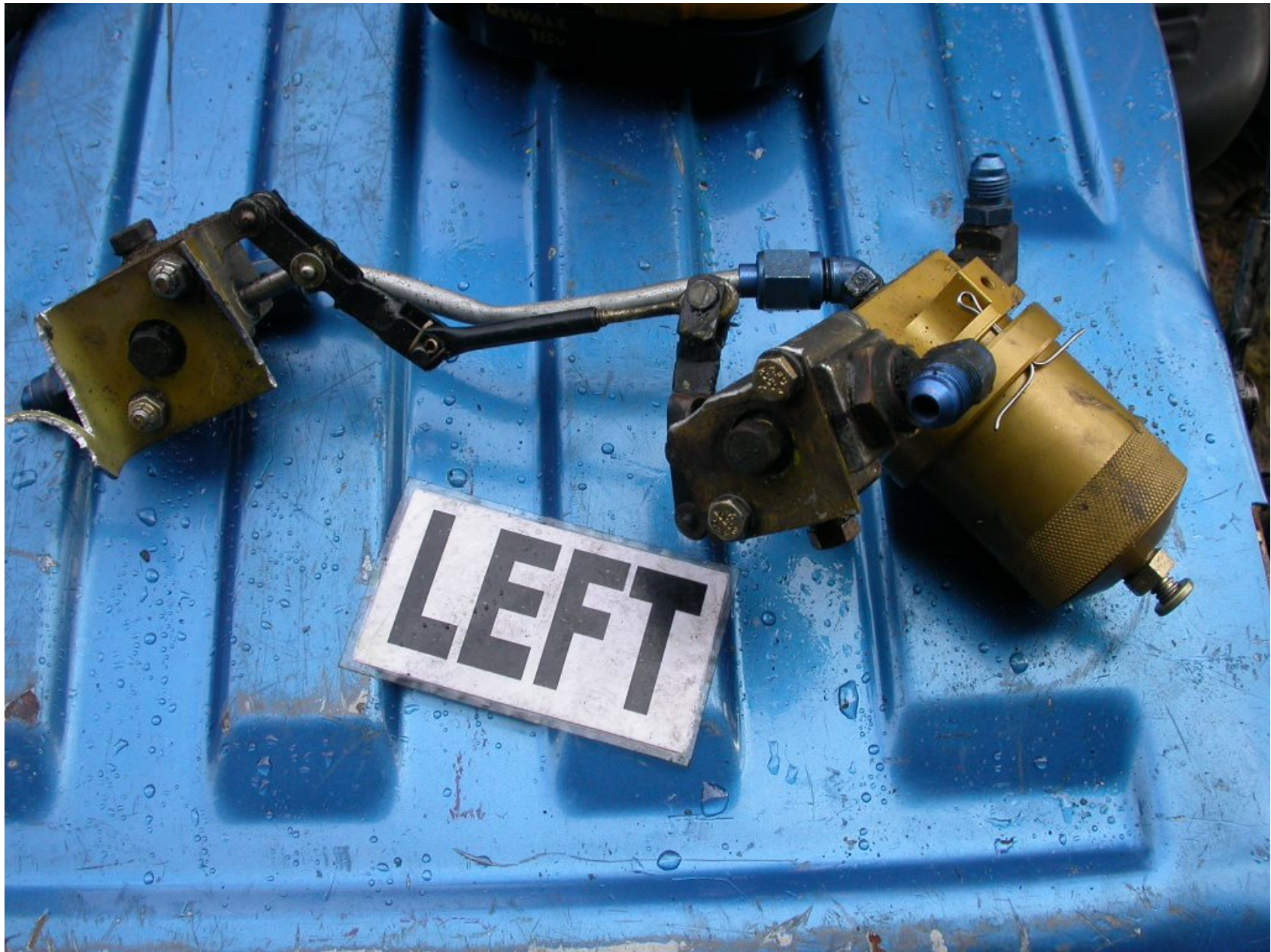
Photo 8 - Left Auxiliary and Main Shutoff Assembly Missing Control Cable
