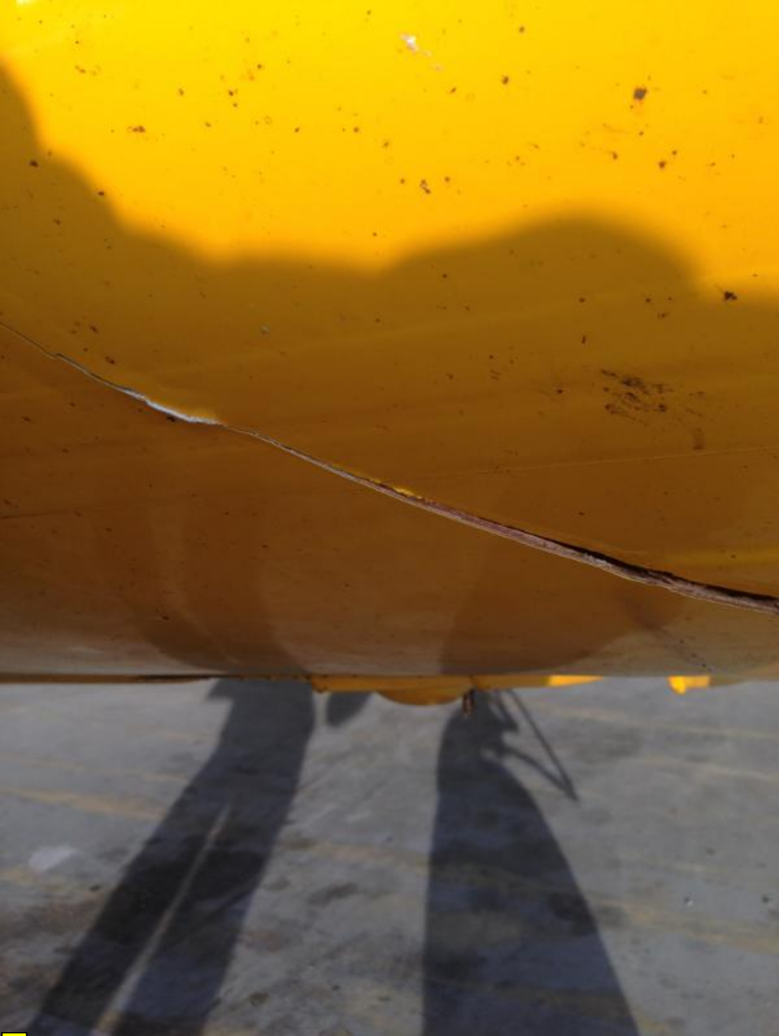
Photo 2 - Damage to Underside of Right Wing (Photo Courtesy of FAA)
