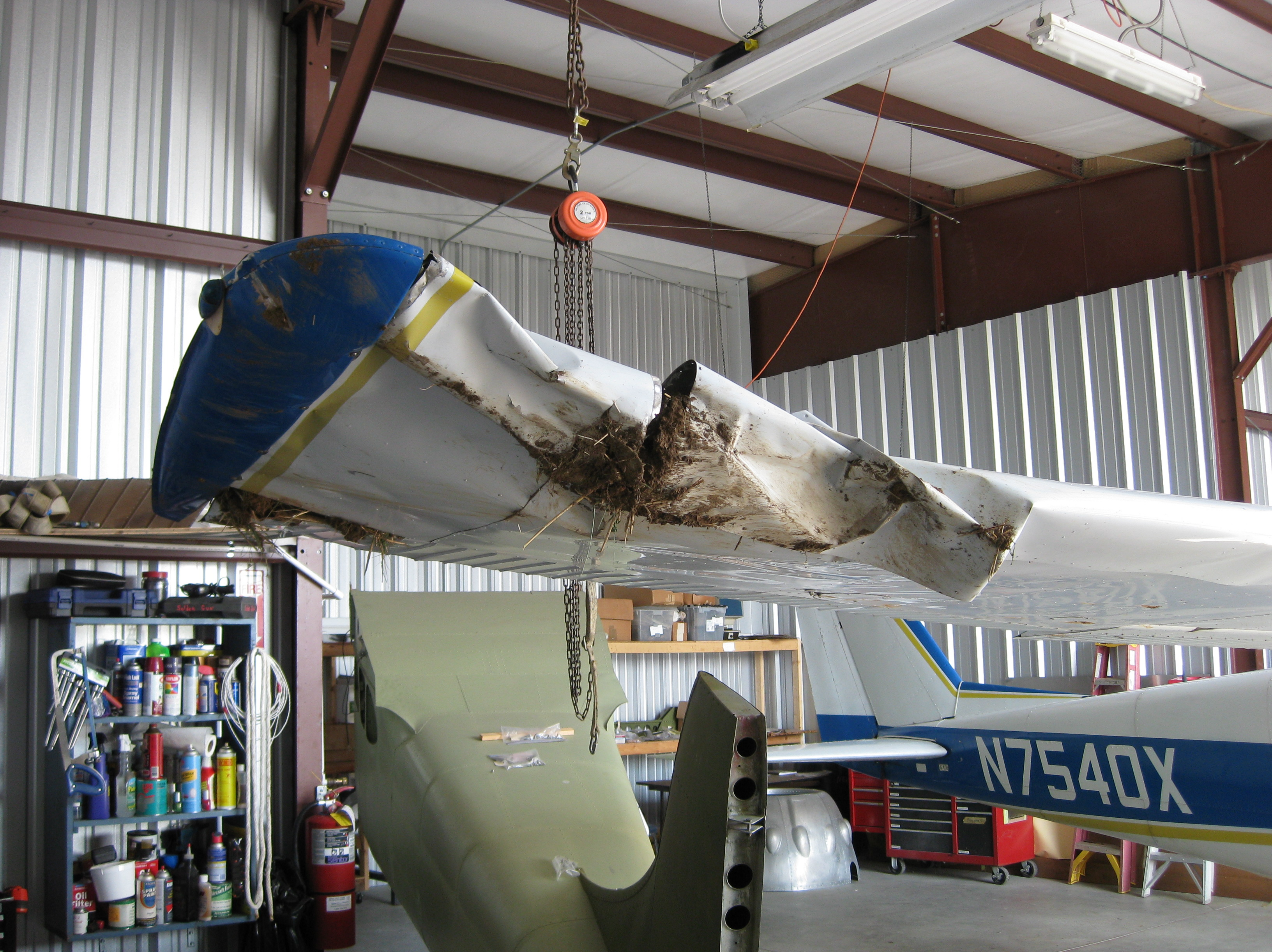
Photo 3 - Outboard Section of Right Wing (Photo Courtesy of FAA)
