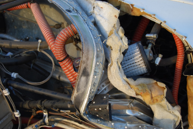
Photo 2. Firewall Damage (Photo Courtesy of [icon])
