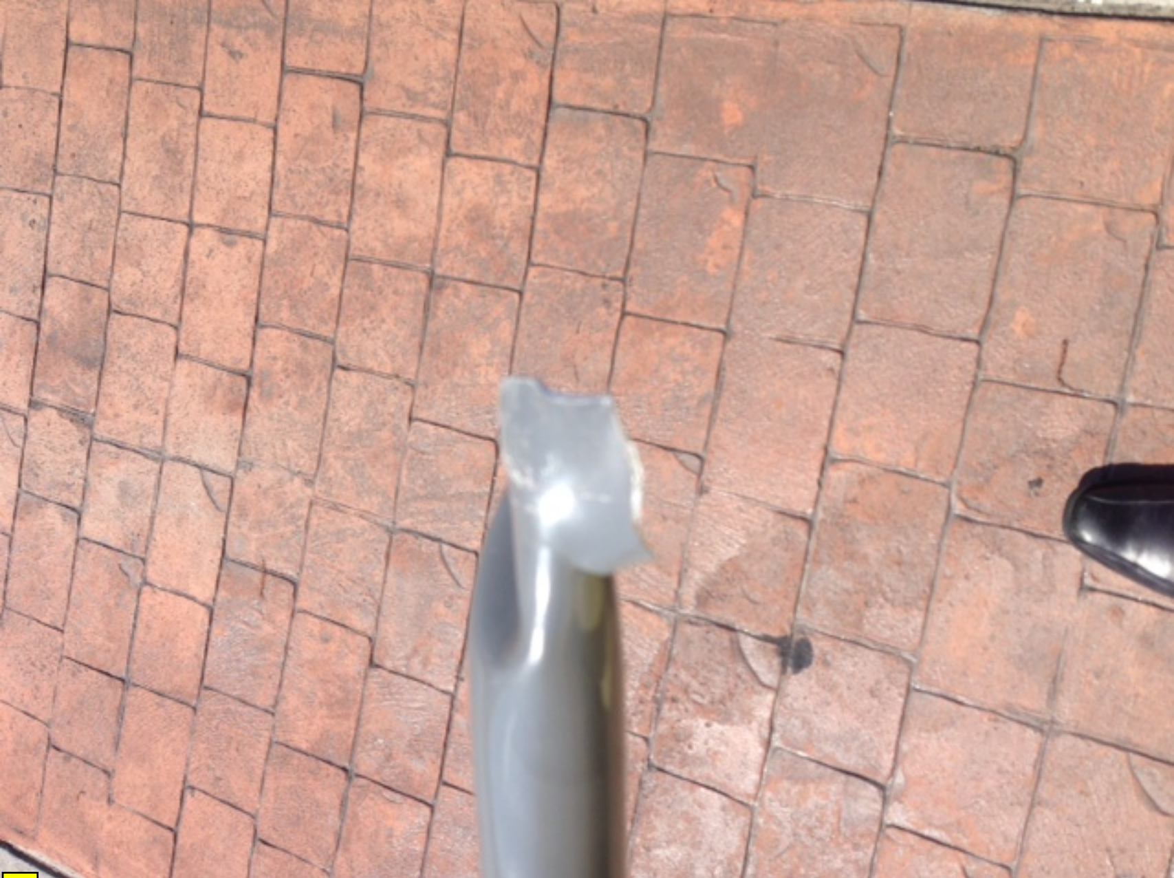
Photo 4. Severed Tail Rotor Drive Shaft End 2 (Photo Courtesy of FAA)
