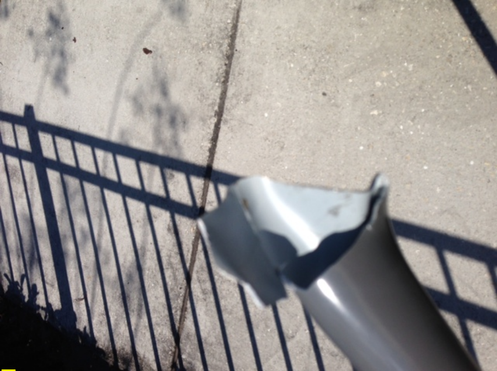
Photo 3. Severed Tail Rotor Drive Shaft End 1 (Photo Courtesy of Air Force Fun Inc.)
