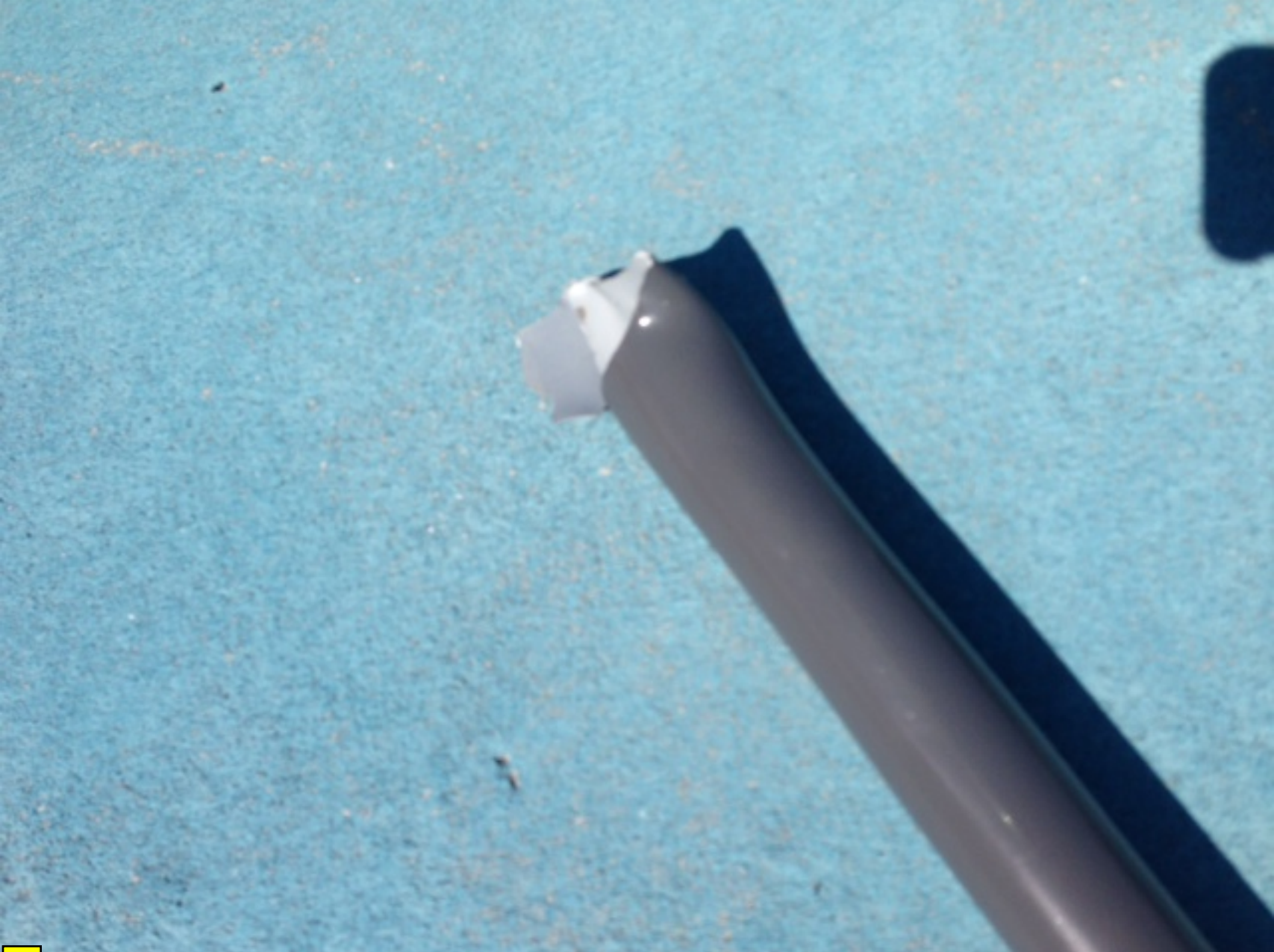
Photo 2. Severed Tail Rotor Drive Shaft (Photo Courtesy of Air Force Fun Inc.)
