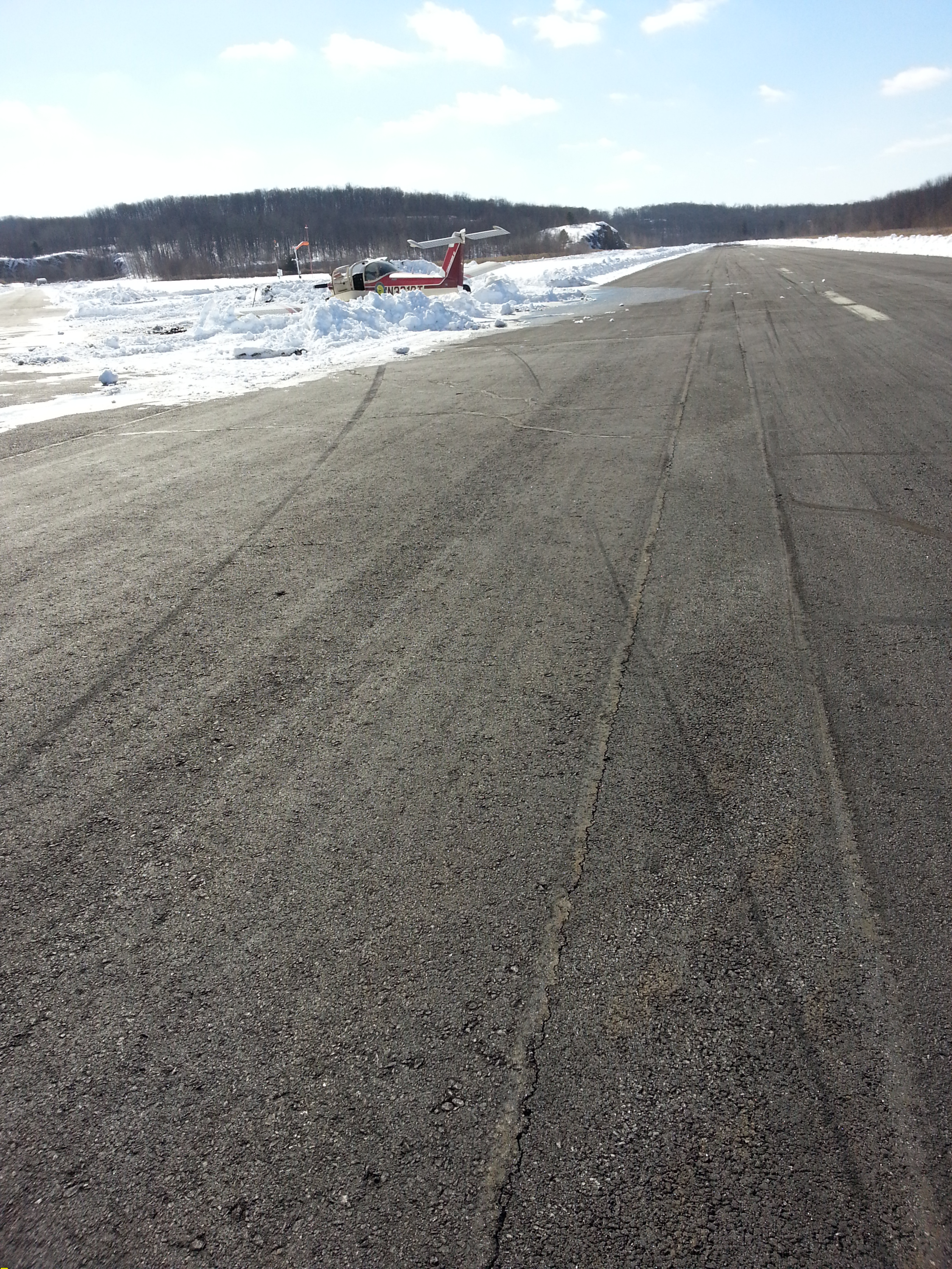
Photo 1. View of Skid Marks on Runway (Digital Photo Courtesy of FAA)
