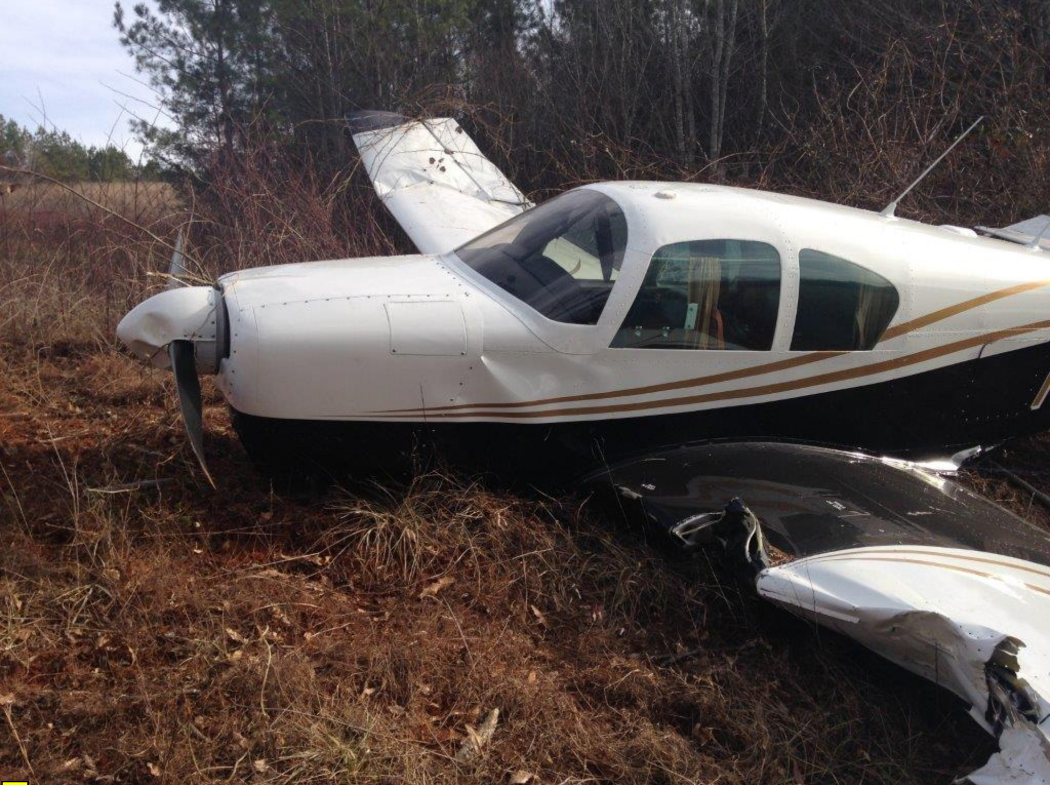
Photo 4. View of Left Wing Damage (photo courtesy of FAA)
