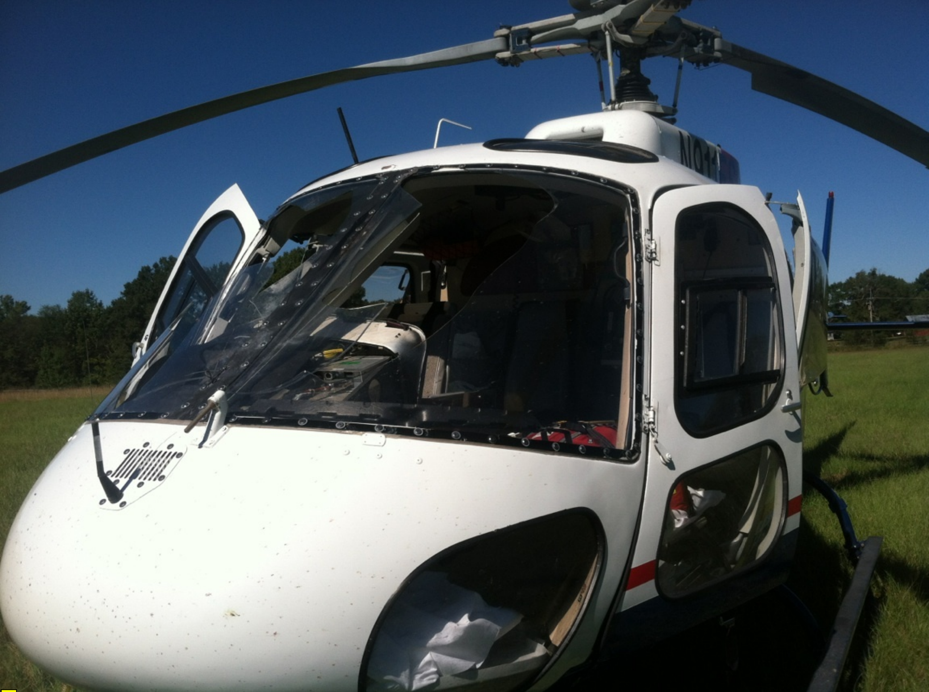
Photo 2 - Helicopter Damage (Courtesy of Operator)
