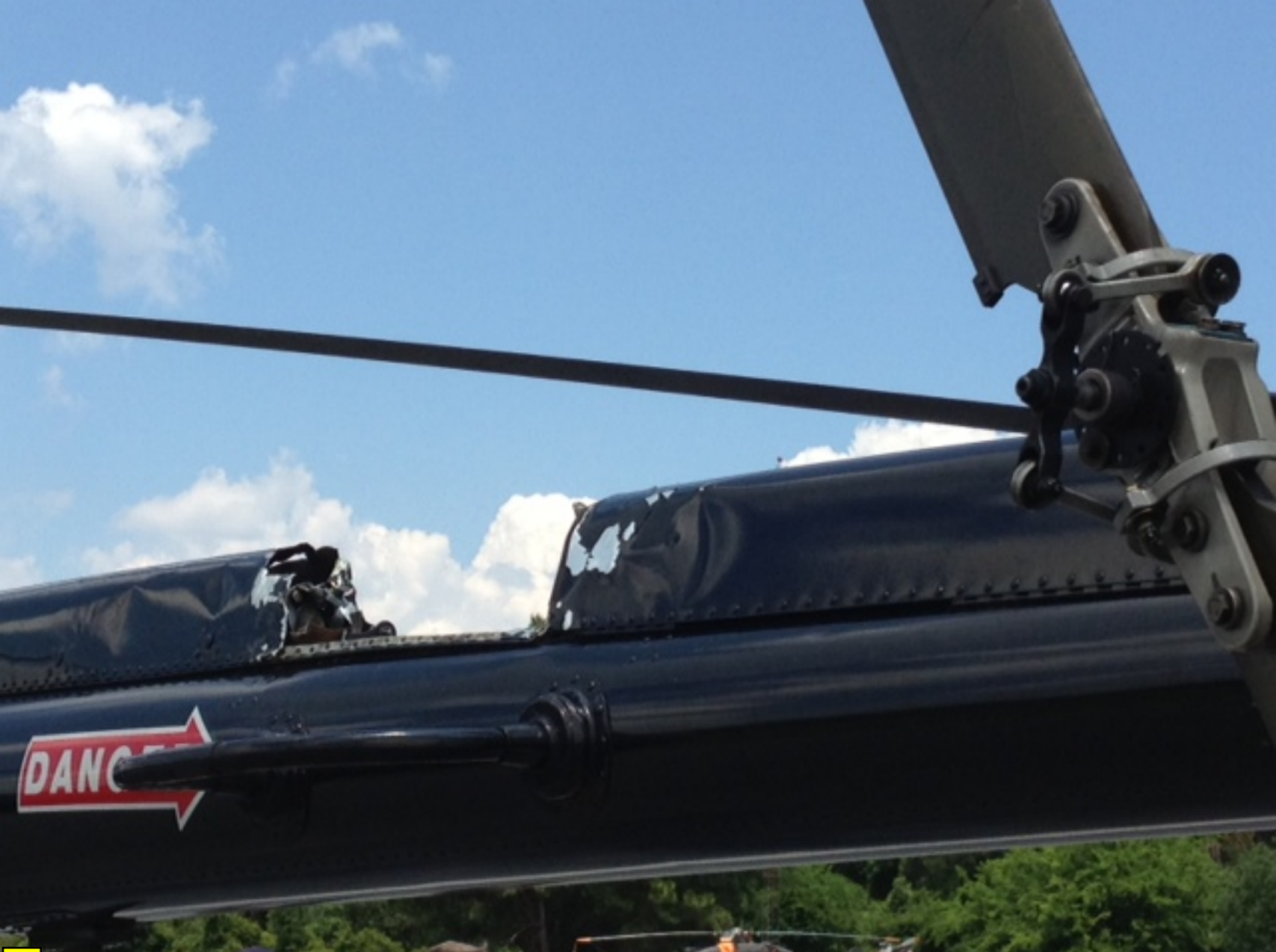
Photo 2 - View of Damage to Tail Rotor Driveshaft Cover and Severed Driveshaft
