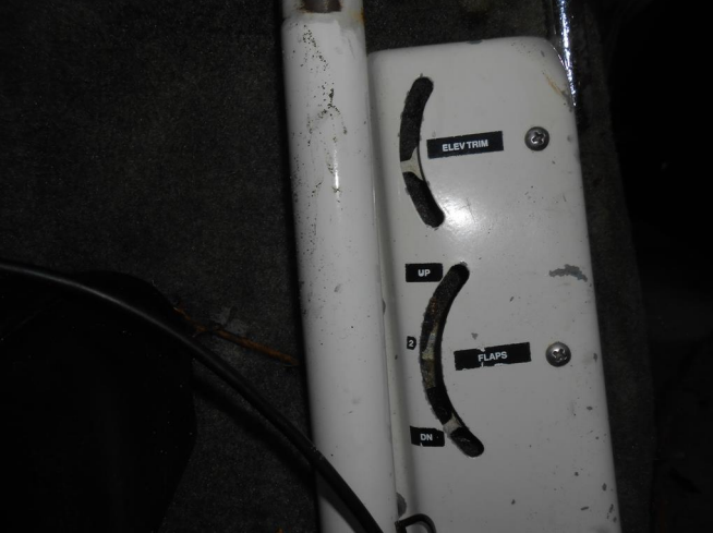
Photograph # 4: Flap Indicator (Photo courtesy of FAA)
