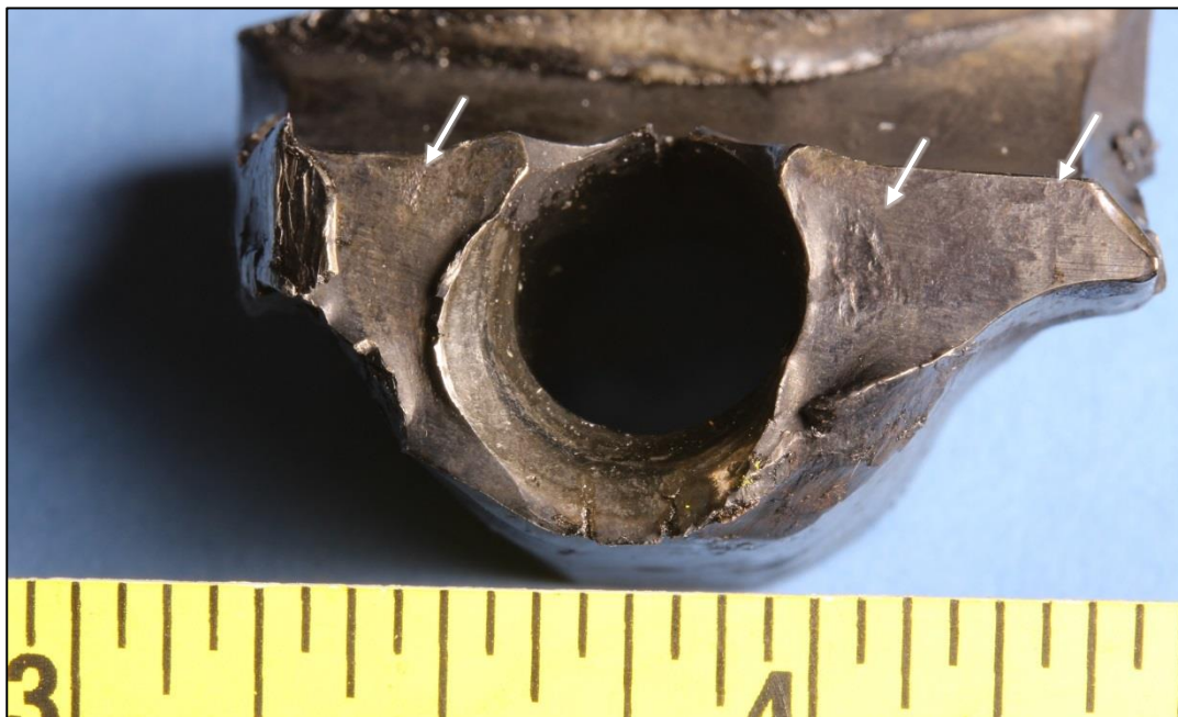
Figure 4. View of the split-line face for the intact strap segment after cutting and cleaning. Arrows indicate areas of fretting damage on the surface.
