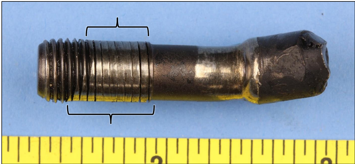
Figure 5. View of the connecting rod bolt piece after removal from the connecting rod and cleaning. Brackets indicate areas of worn thread peaks.
