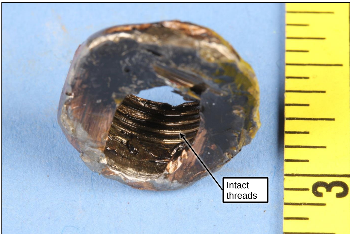
Figure 6. Close view of the connecting rod nut showing intact internal threads.
