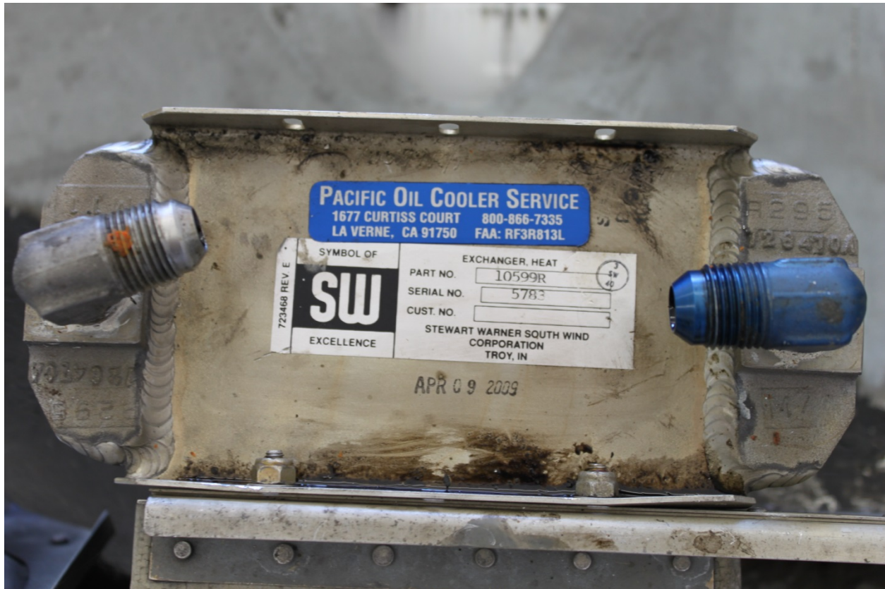
Photo 24: Oil Cooler/Heat Exchanger
