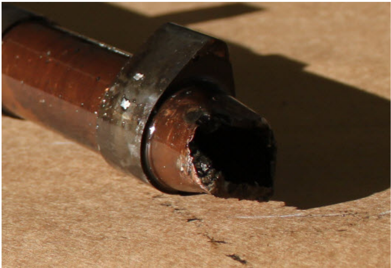
Photo 14: Fracture Surface of the Camshaft
