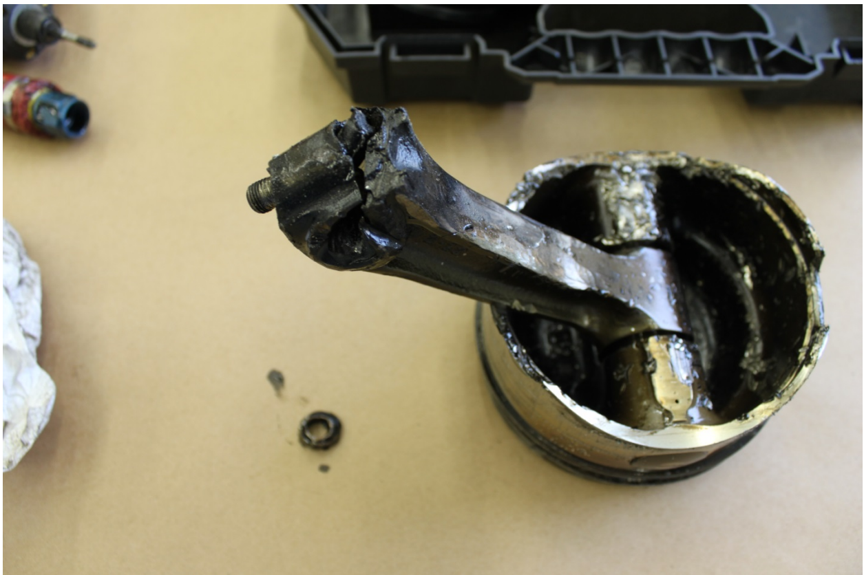
Photo 11: Cylinder No. 6 Arm with Bolt attached and Nut found in the Bottom of the Oil Pan
