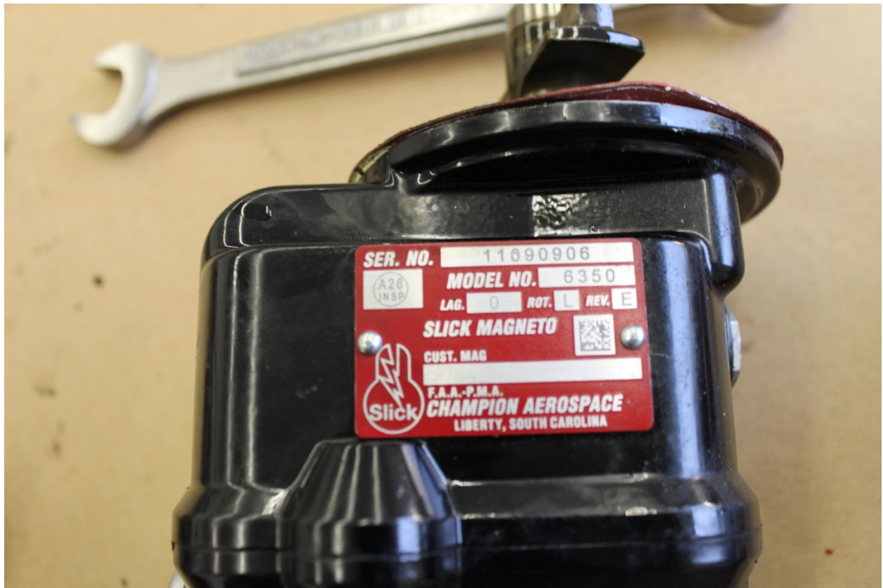
Photo 20: Right Magneto after Removal
