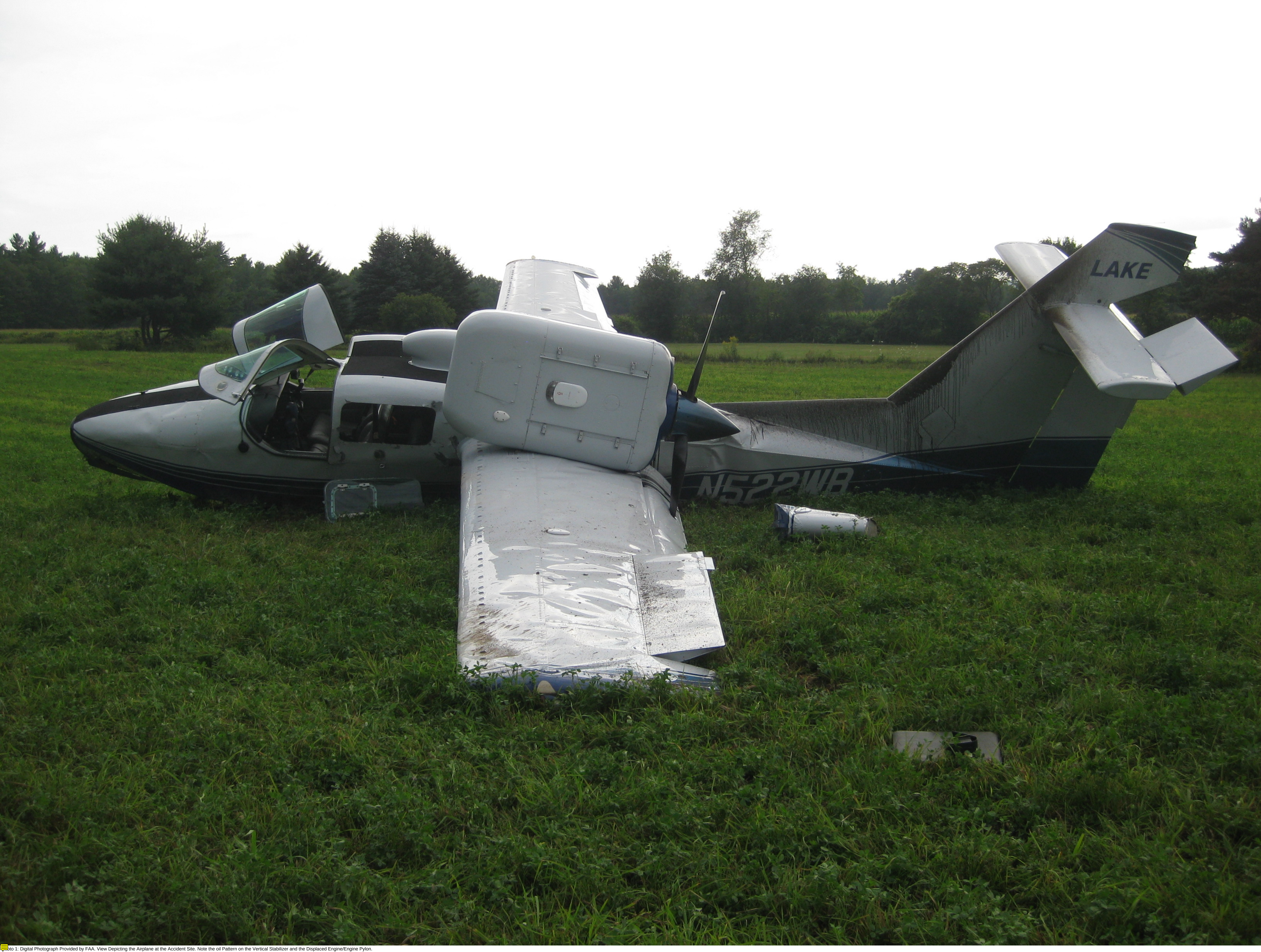
Photo 1: Digital Photograph Provided by FAA. View Depicting the Airplane at the Accident Site. Note the oil Pattern on the Vertical Stabilizer and the Displaced Engine/Engine Pylon.
