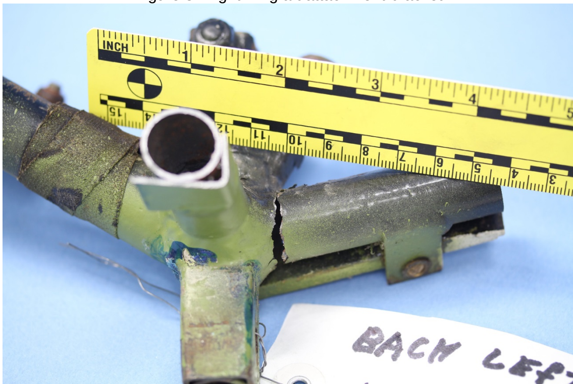
Figure 4: Left wing aft attachment bracket with fracture at the weld
