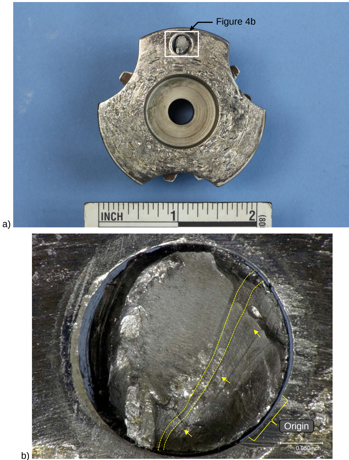
Figure 4: a) Image of the face of the crankshaft gear that mates with the face of the counterbored pilot hole and b) image of the fractured alignment dowel. Crack arrest marks were observed and the fracture had a flat appearance, consistent with a fatigue fracture. The piece of the dowel rotated approximately 180° after it fractured.
