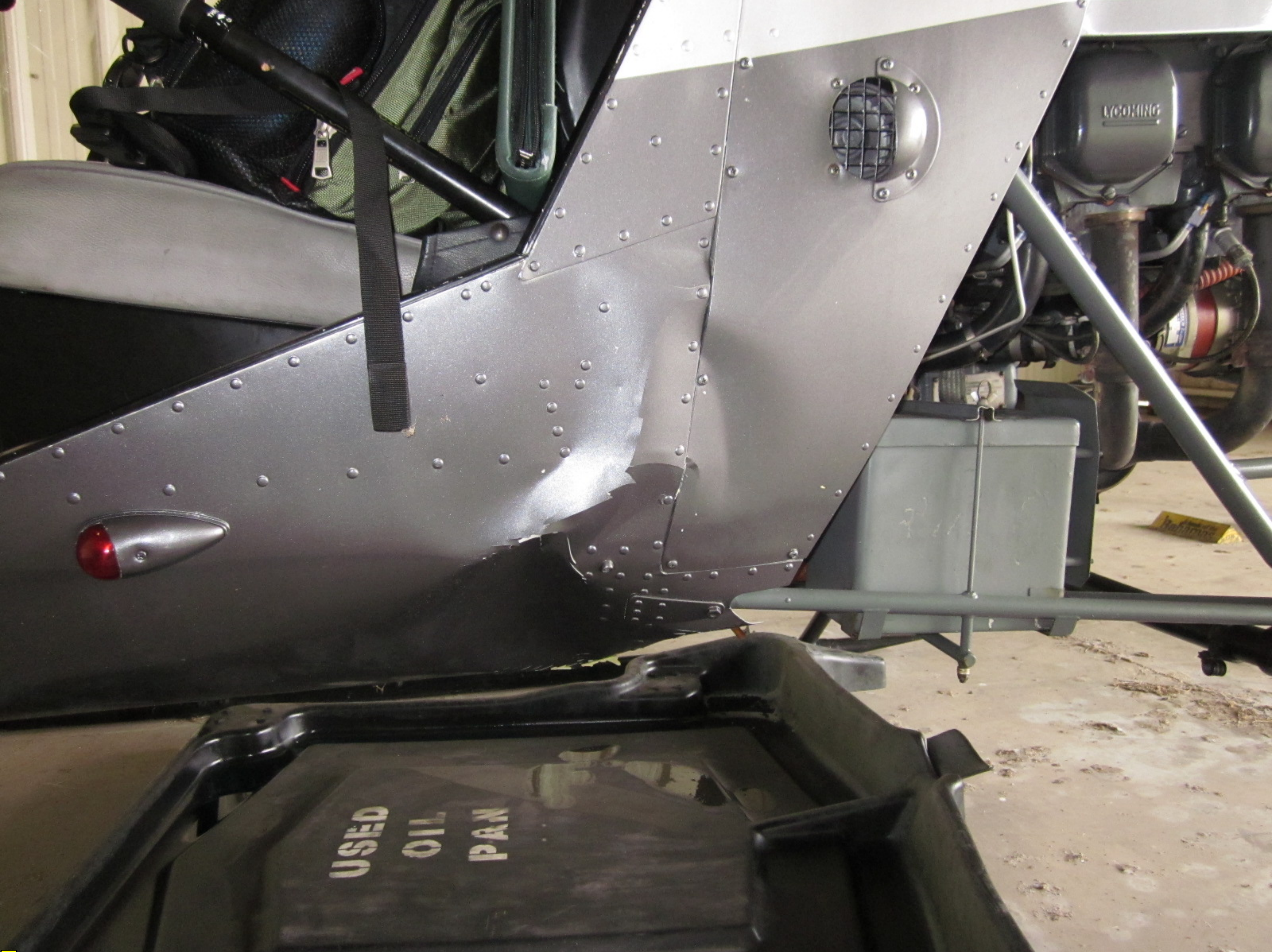
Photo 2: Fuselage Buckling (FAA Digital Photo)
