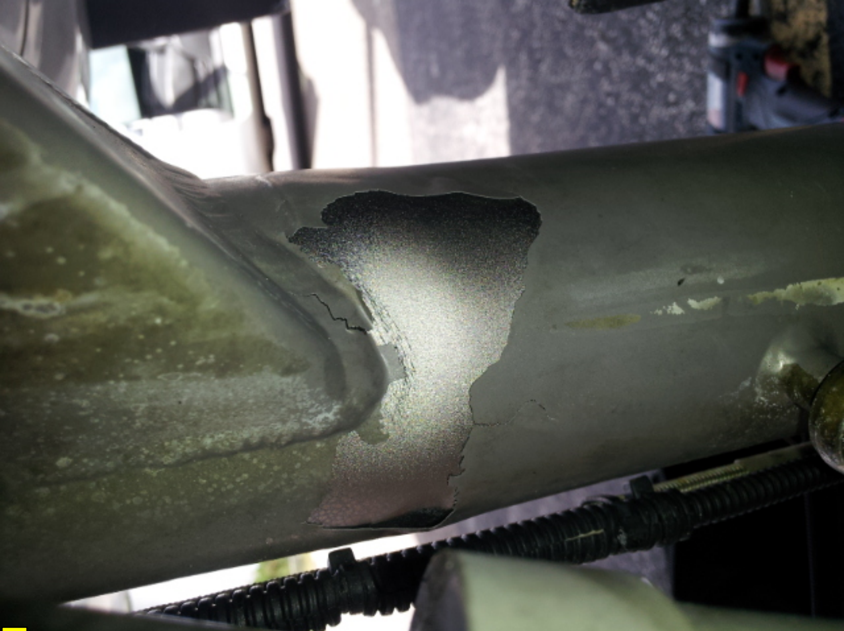
Photo 3-Over stressed trunion (FAA)
