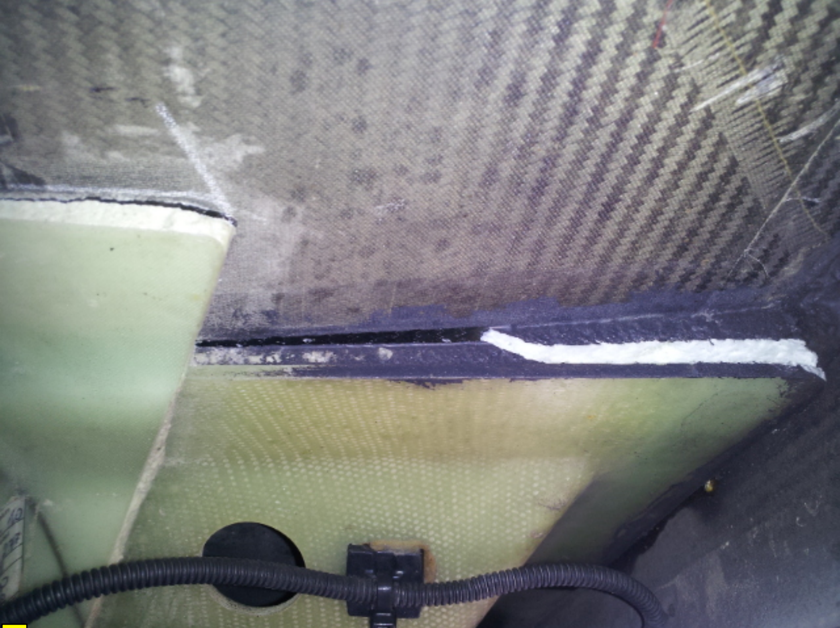
Photo 2-wing spar fractured at the fuselage bulkhead (FAA)
