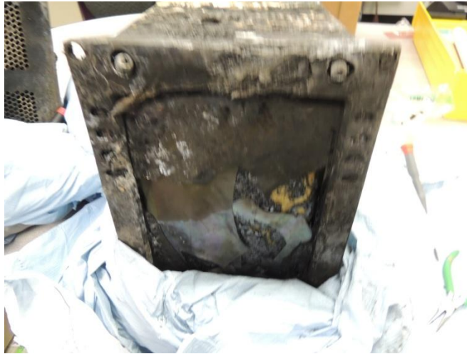
Figure 4. Avidyne PCB containing two flash memory chips recovered from PFD.
