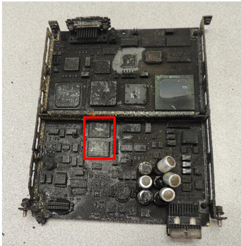
Figure 4. Avidyne PCB containing two flash memory chips recovered from PFD.
