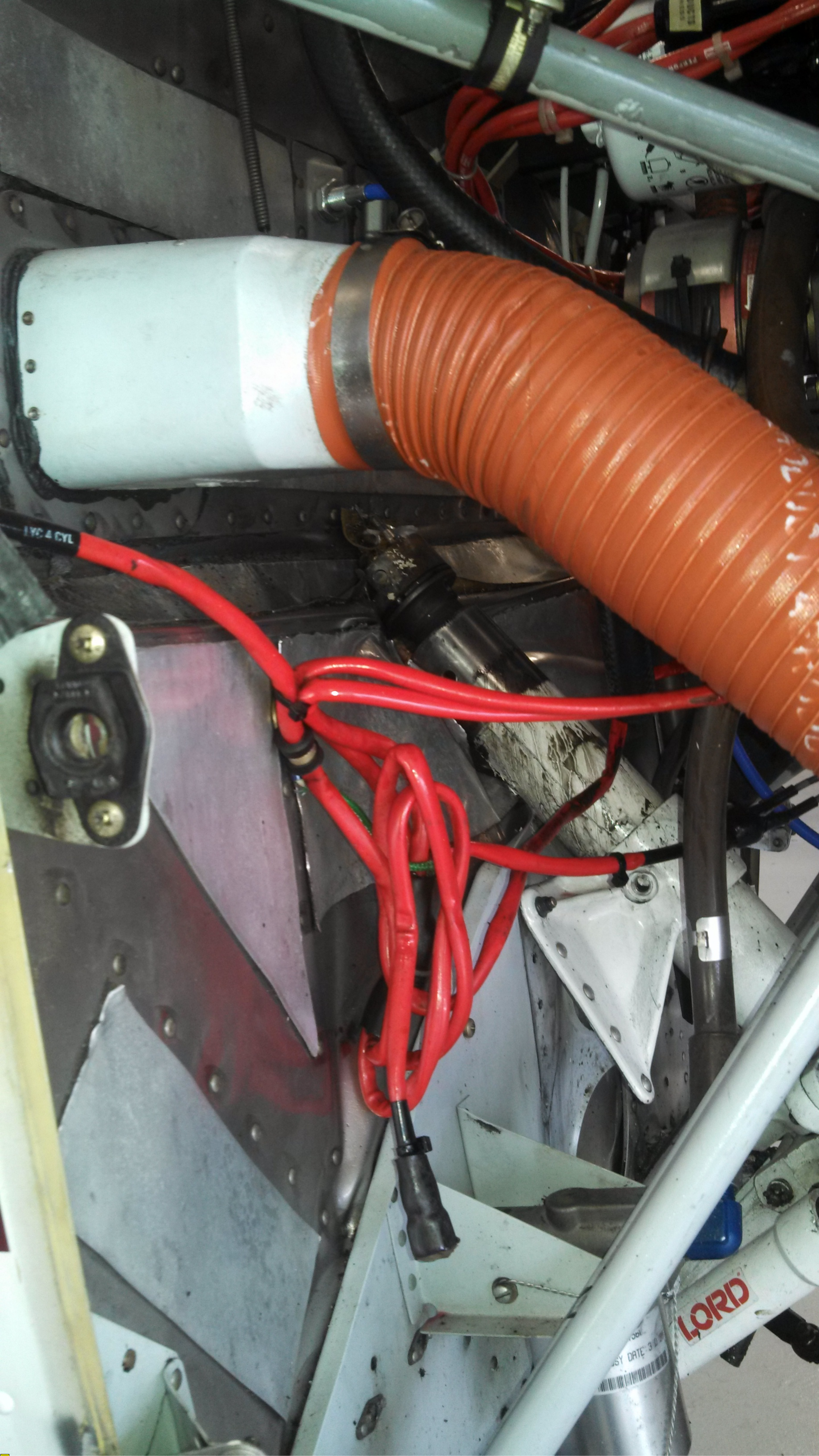
Photo 2: Damage to engine firewall.(Courtesy of the FAA)
