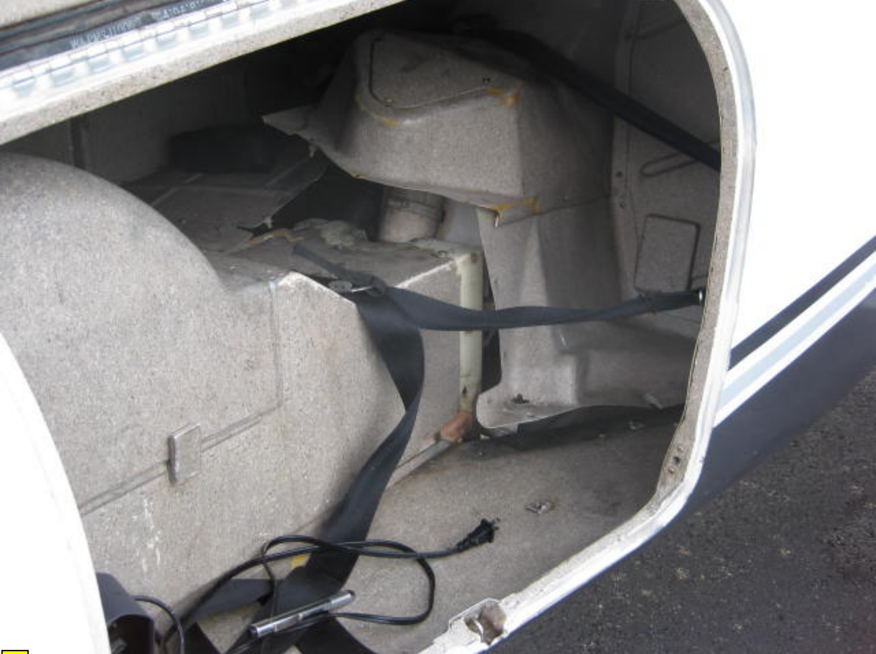
Photo 4-Courtesy of FAA-View of inside baggage compartment showing damaged forward bulkhead and nose trunnion
