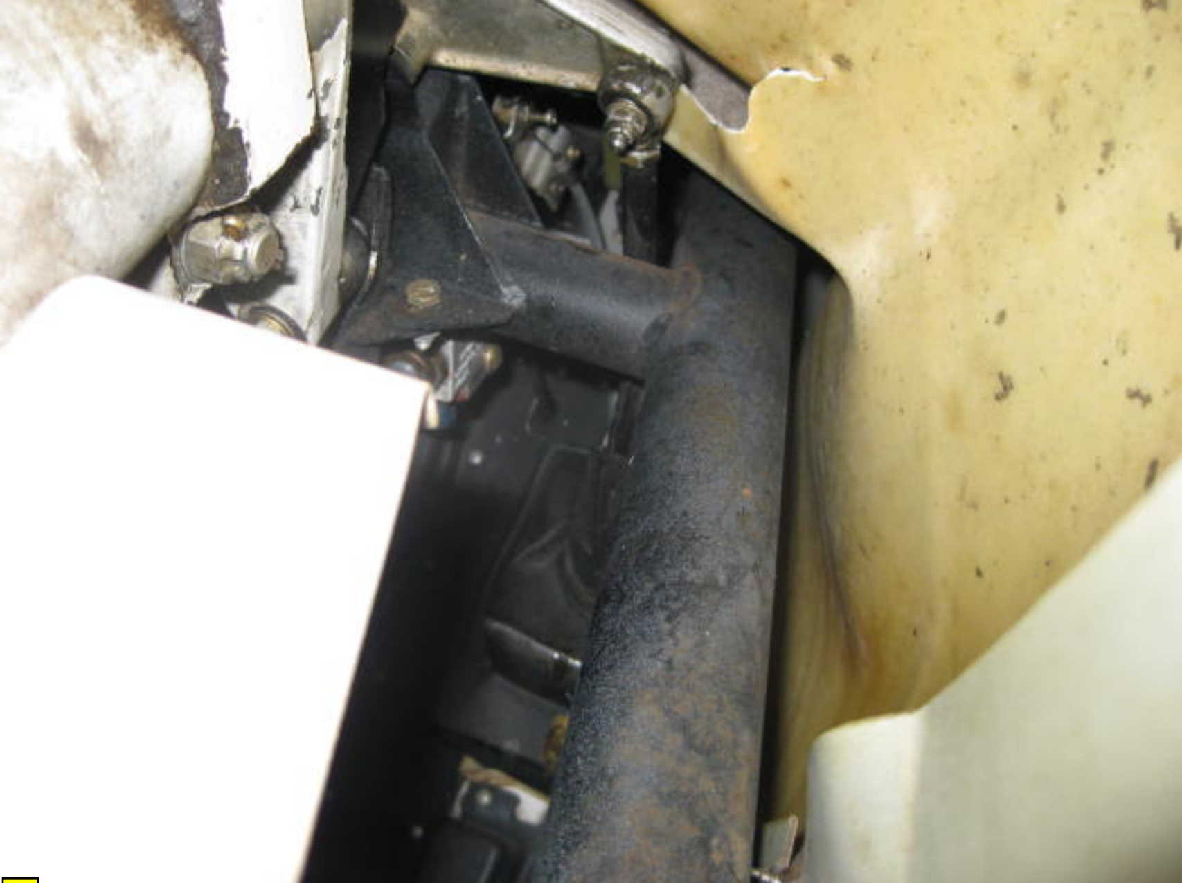
Photo 2-Courtesy of FAA-View of landing gear assembly and buckled firewall
