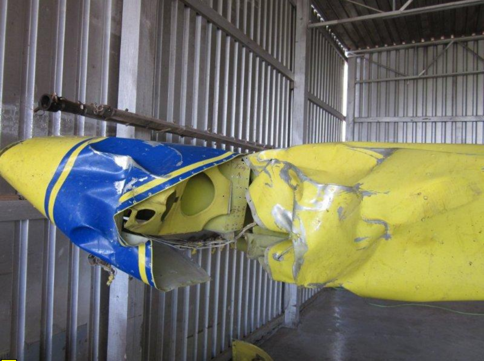
Photo 2 - Damage to Right Wing Tip (Photo Courtesy of FAA)
