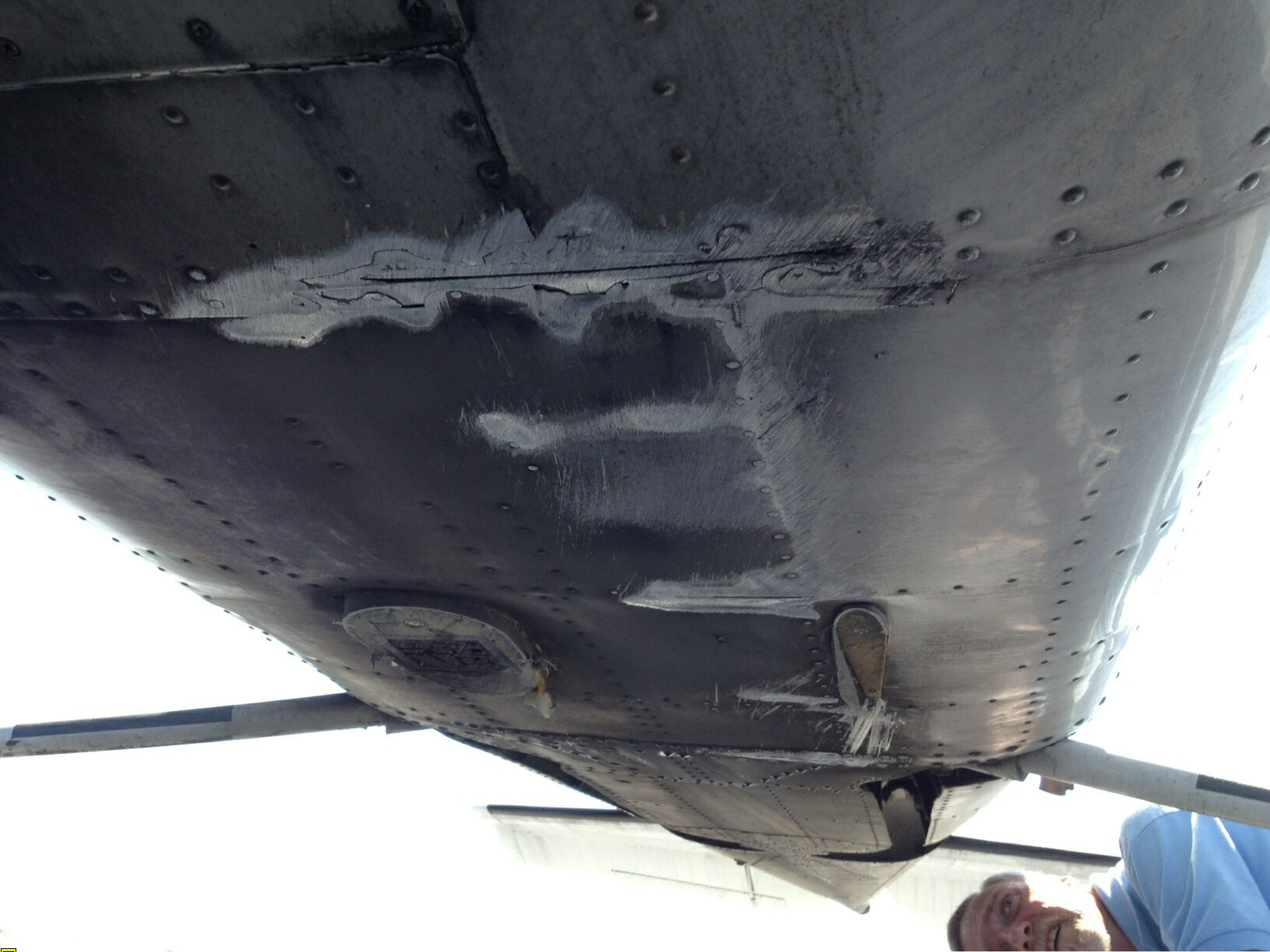
Photo 1: Damage to underside of fuselage (Courtesy of FAA)
