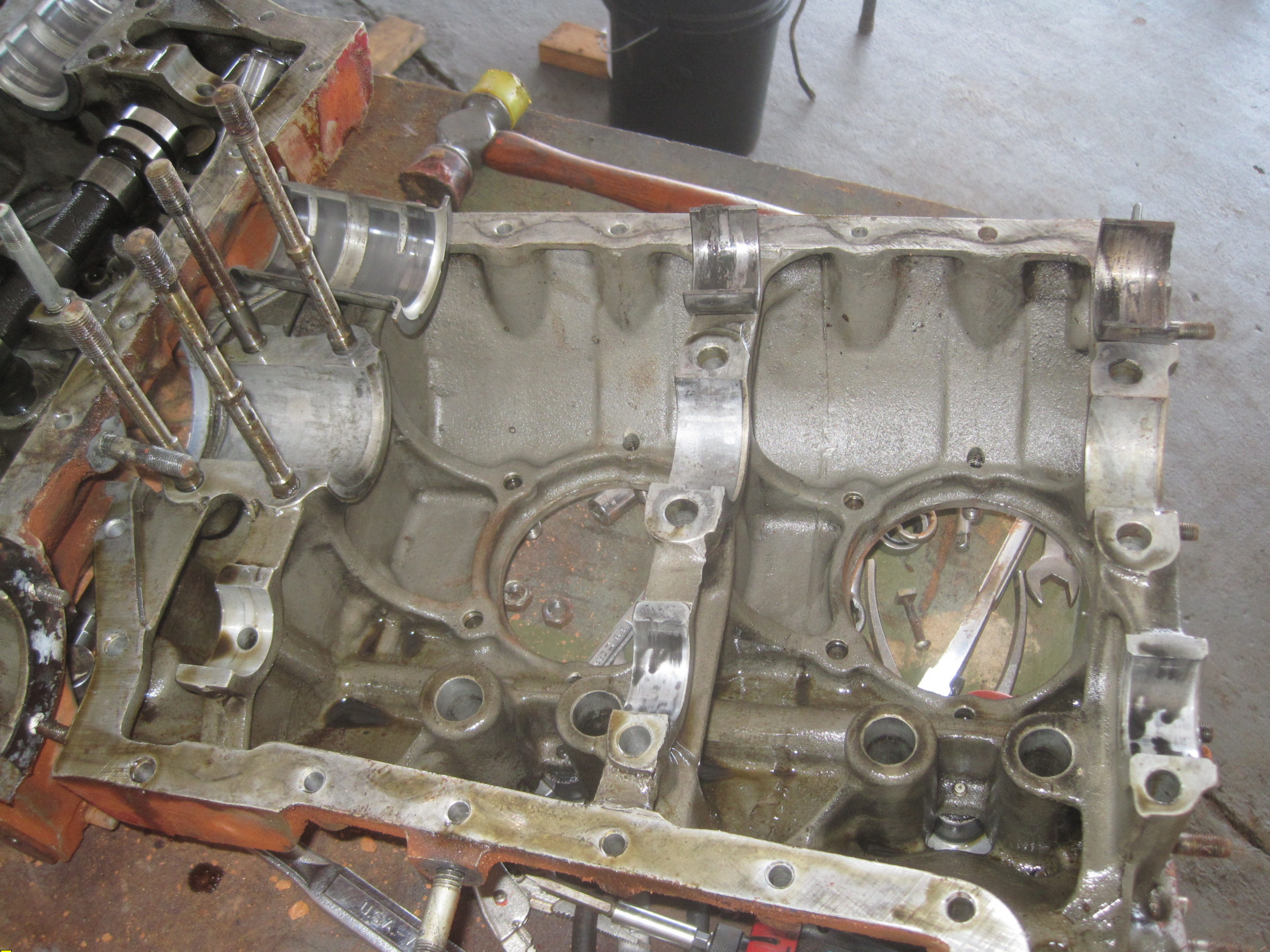
Photo 5) View of crankshaft and camshaft bearings. Photo provided by FAA.
