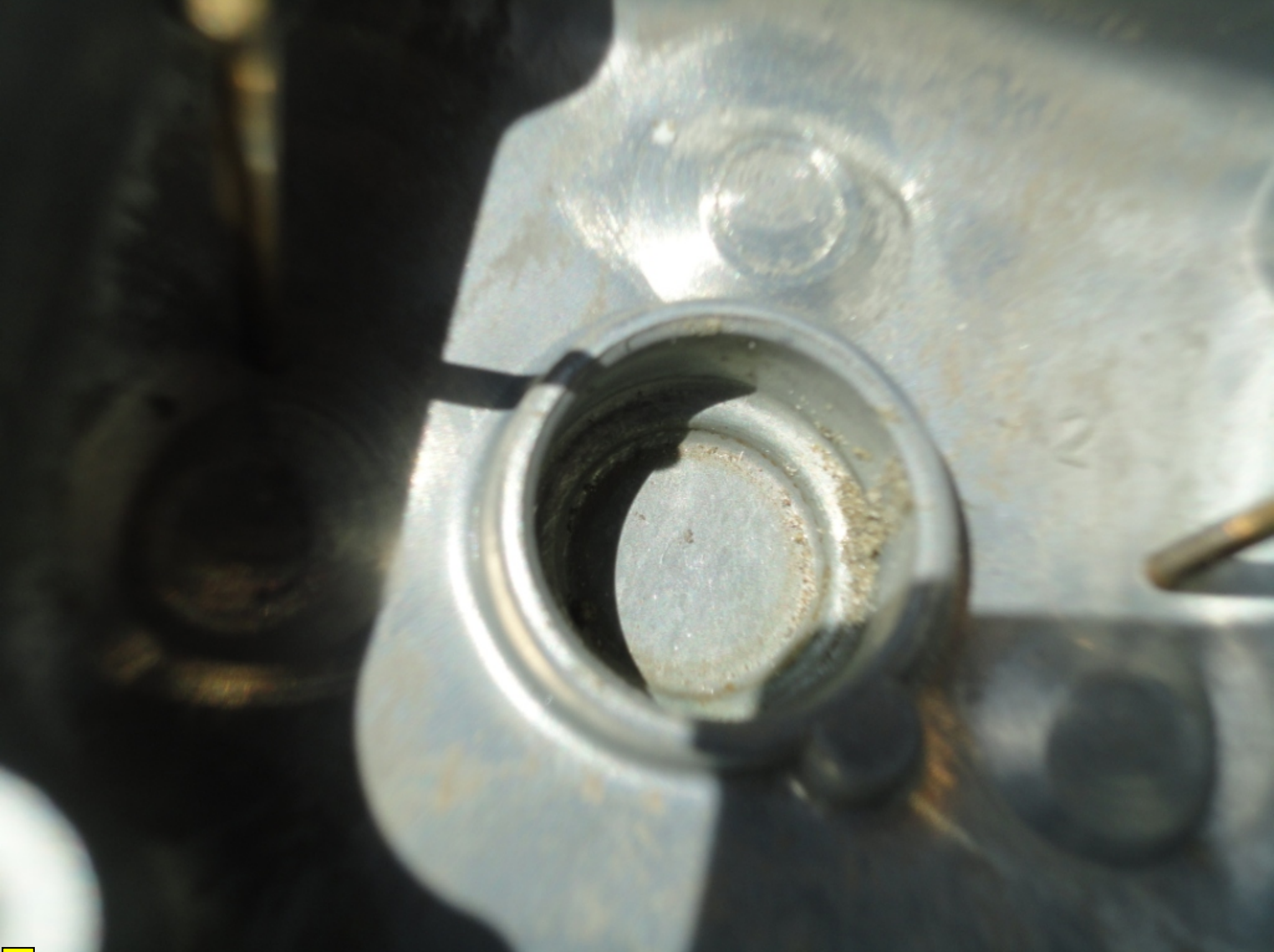
Photo 4 - Particulate Found Inside Left Carburetor (Photo Courtesy of Rotech)
