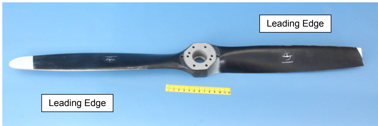
Figure 1. An overall view of the chamber side of the as-received propeller with the fracture at the right.
