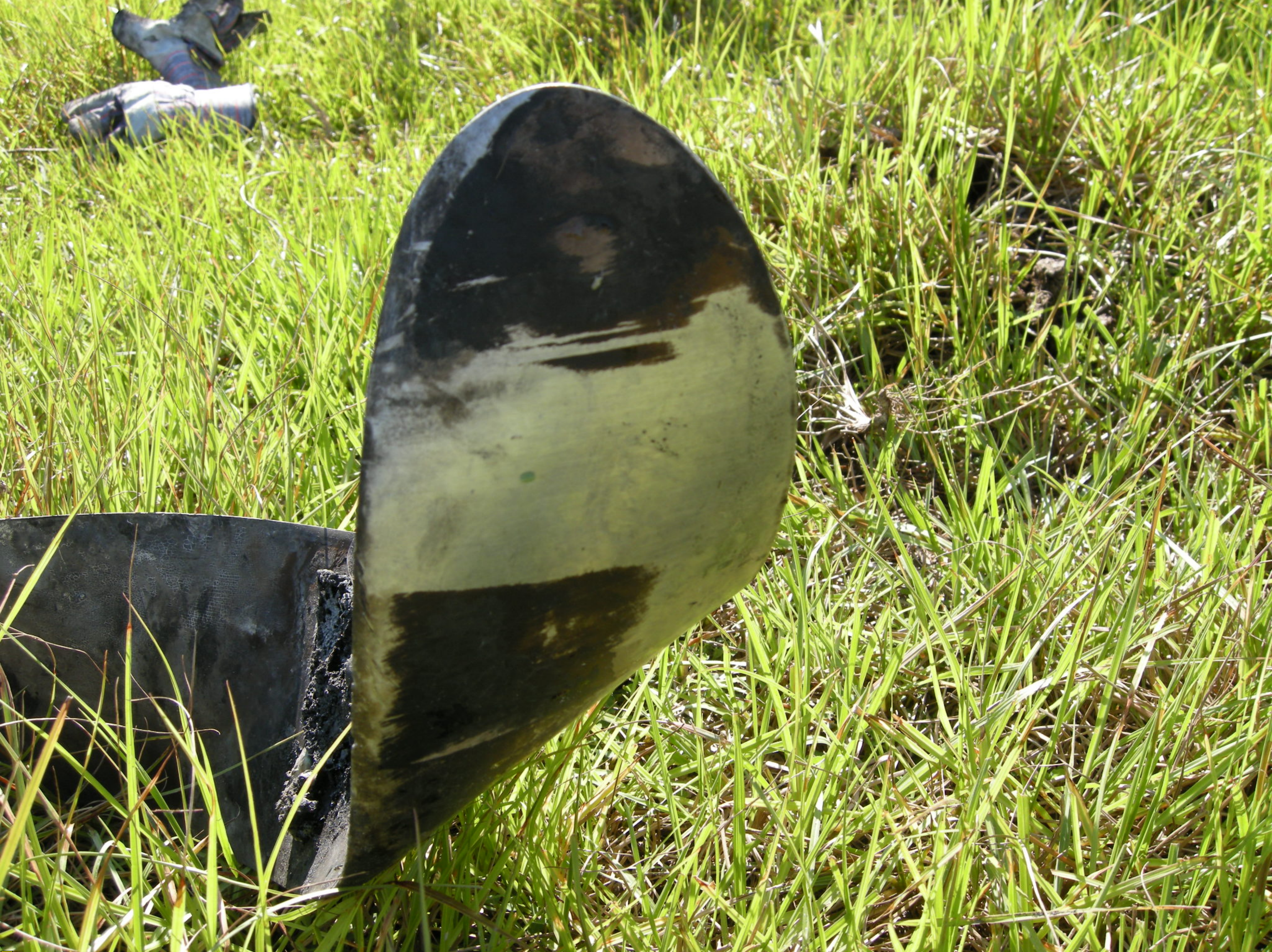
Photo 9: Propeller Tip, with Chordwise Scratches and Surface Polishing. NTSB Digital Photo.
