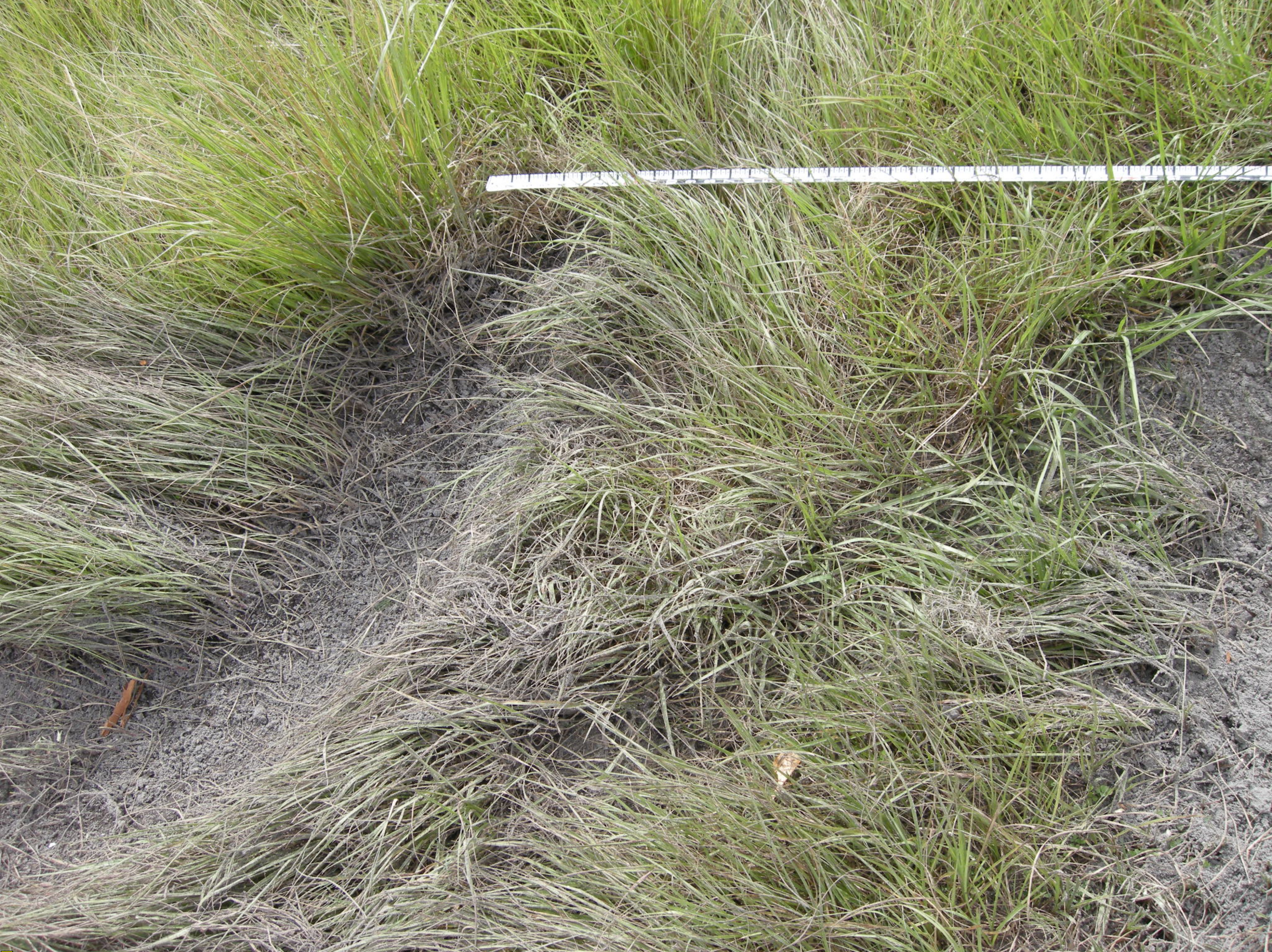
Photo 4: Slash Marks Found at Area of Initial Ground Impact. NTSB Digital Photo.
