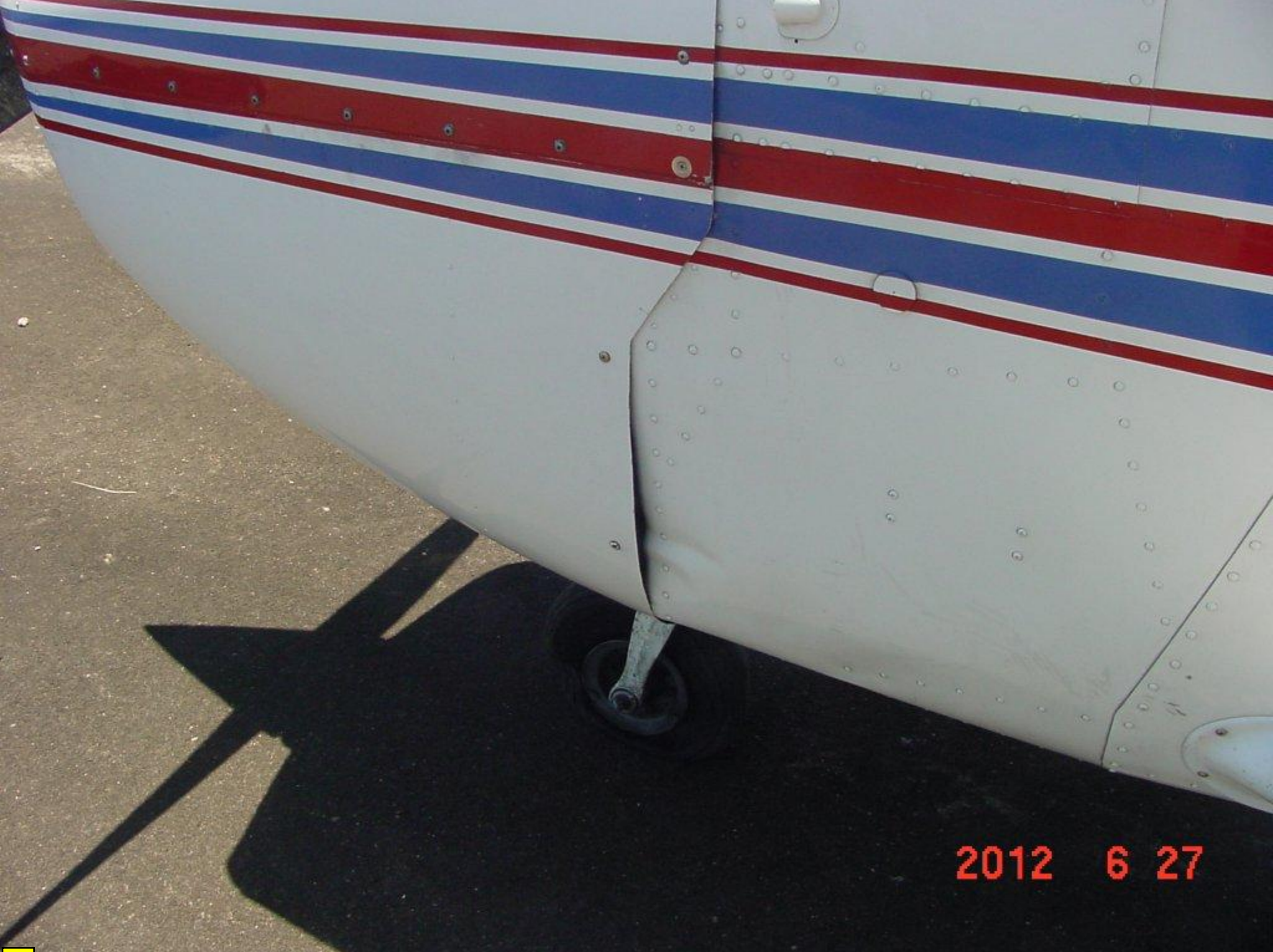
Photo 1: View of Fuselage Damage (Courtesy of FAA)
