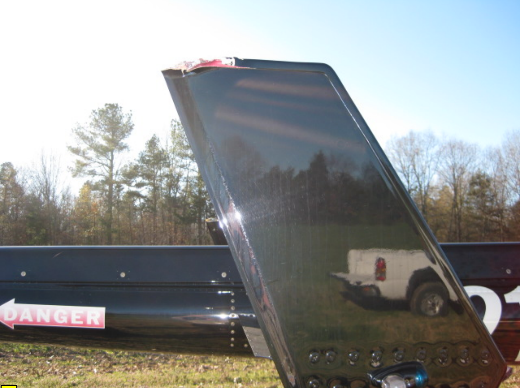
Photo 4 - Damage to Left Vertical Stabilizer (Courtesy FAA)
