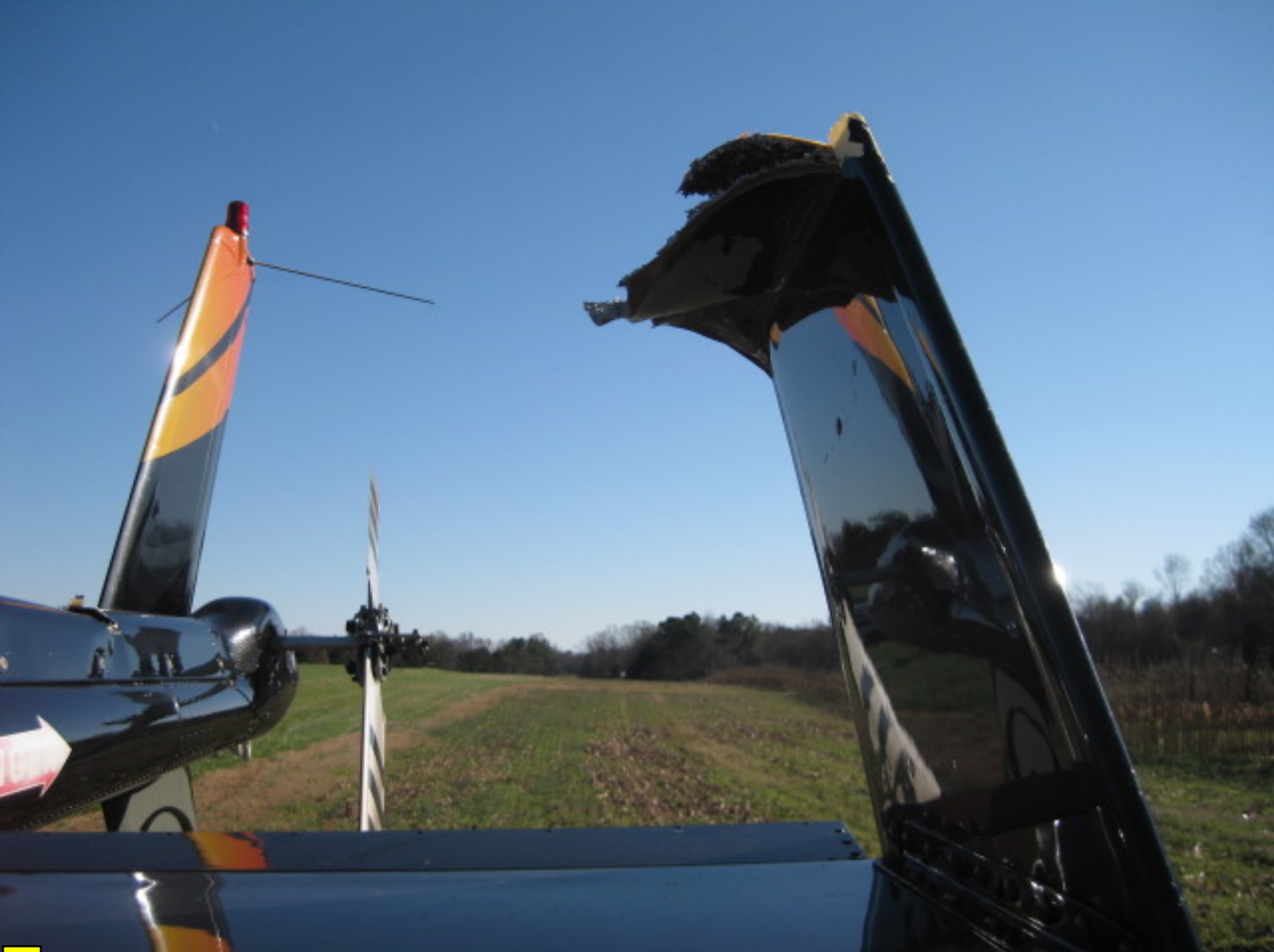
Photo 3 - Damage to Right Vertical Stabilizer (Courtesy FAA)
