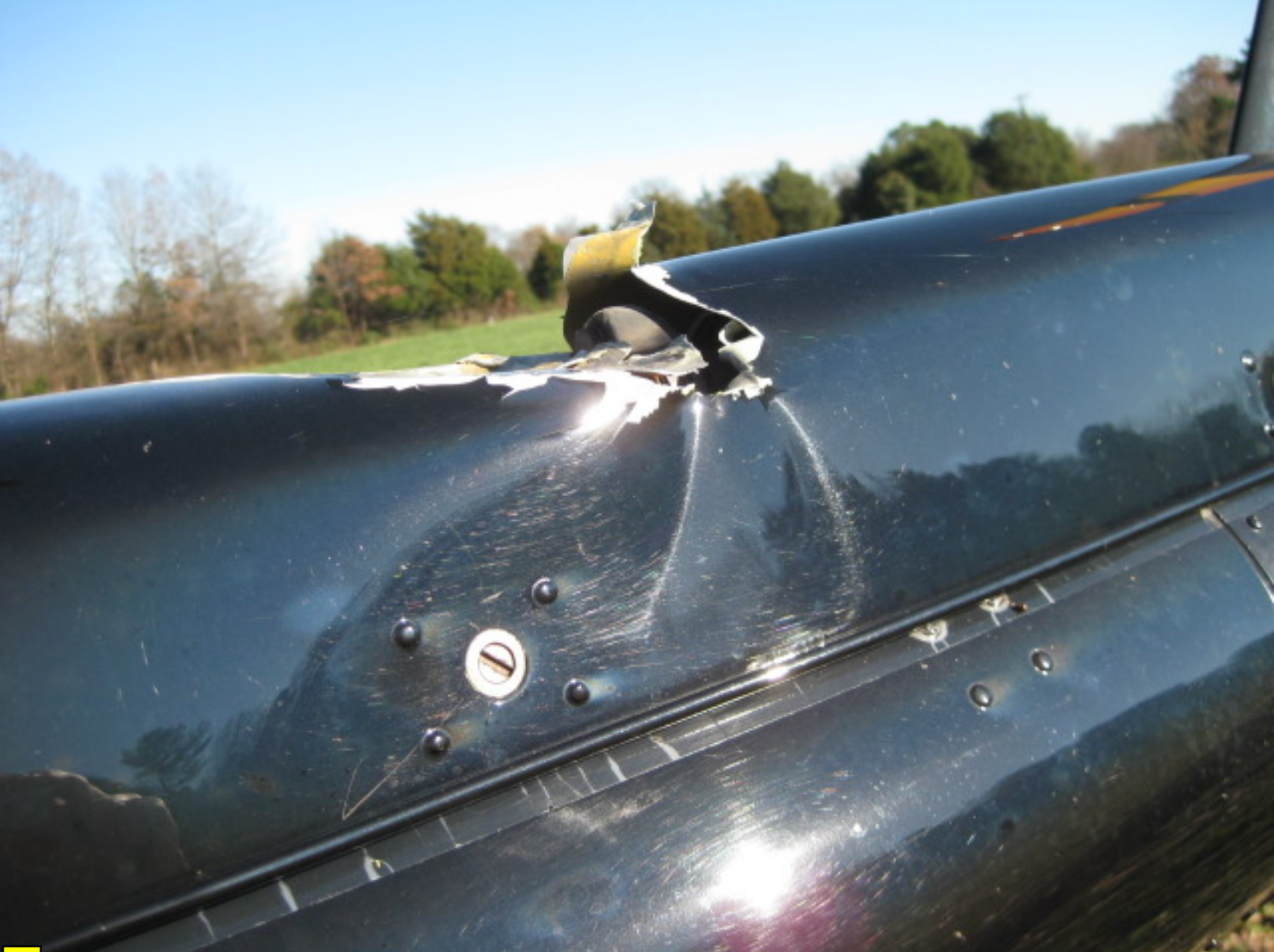
Photo 1 - Damage to Tail Rotor Drive Shaft Cover(Courtesy FAA)
