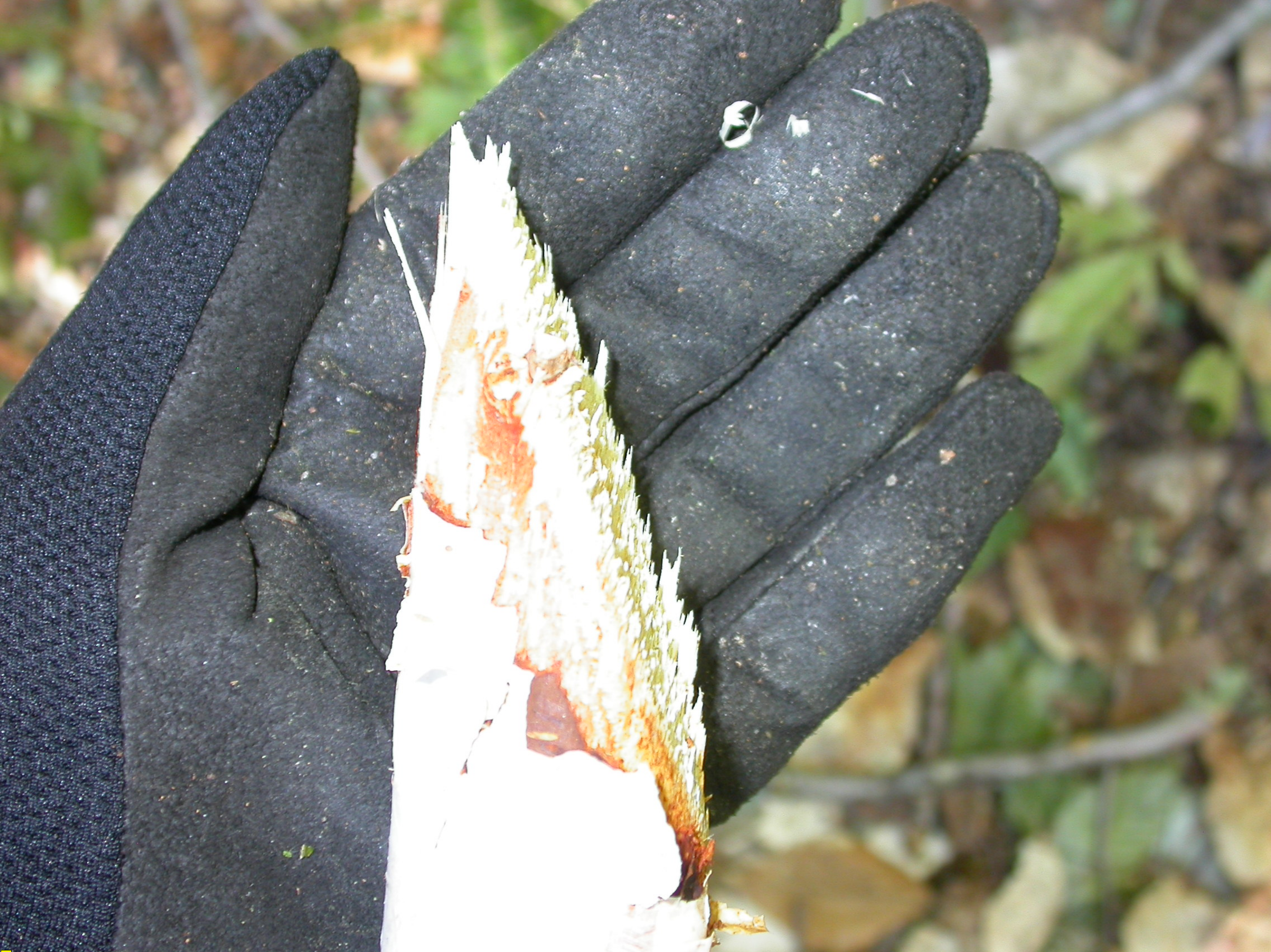
Photo 6: Photograph of Propeller Strike Mark on Tree Limb
