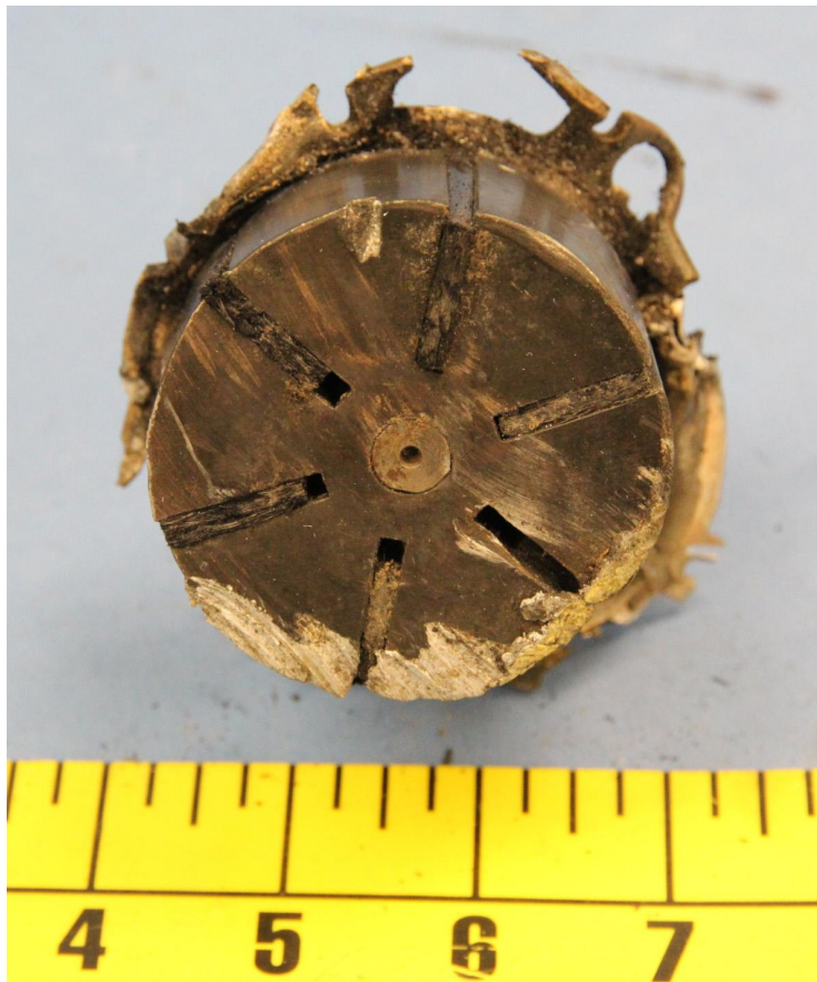
Figure 3. The intact gimbal structure with gyro disassembled.
