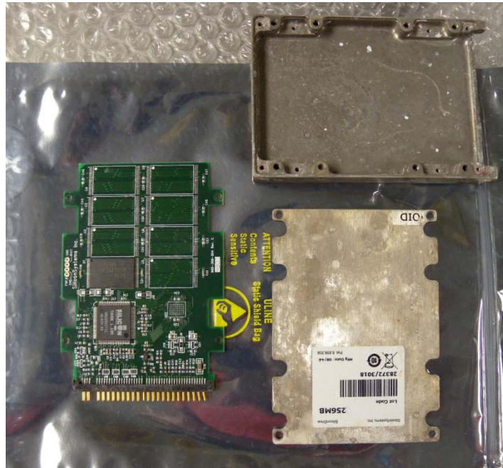
Figure 1 - Solid State Hard Drive removed from Avidyne 750 MFD
