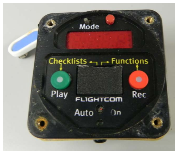
Figure 4 - Flightcom DVR 300i as received (note: external battery is disconnected)
