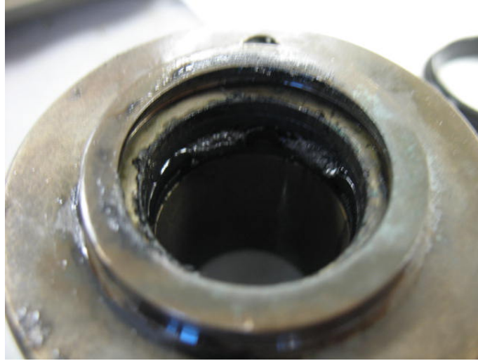
Photo 3. T-Seal in Groove Showing "Rolling Phenomenon" (Courtesy of Triumph Actuation Systems)
