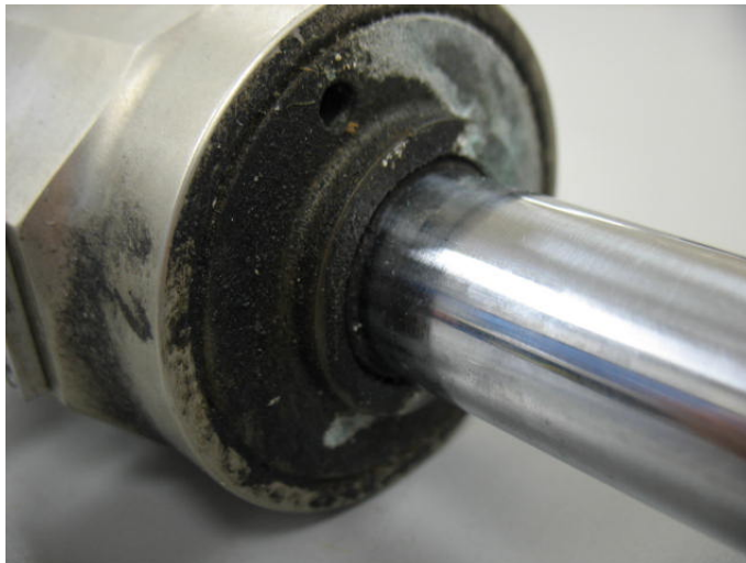
Photo 2. Corrosion on scraper faceplate (Courtesy of Triumph Actuation Systems)
