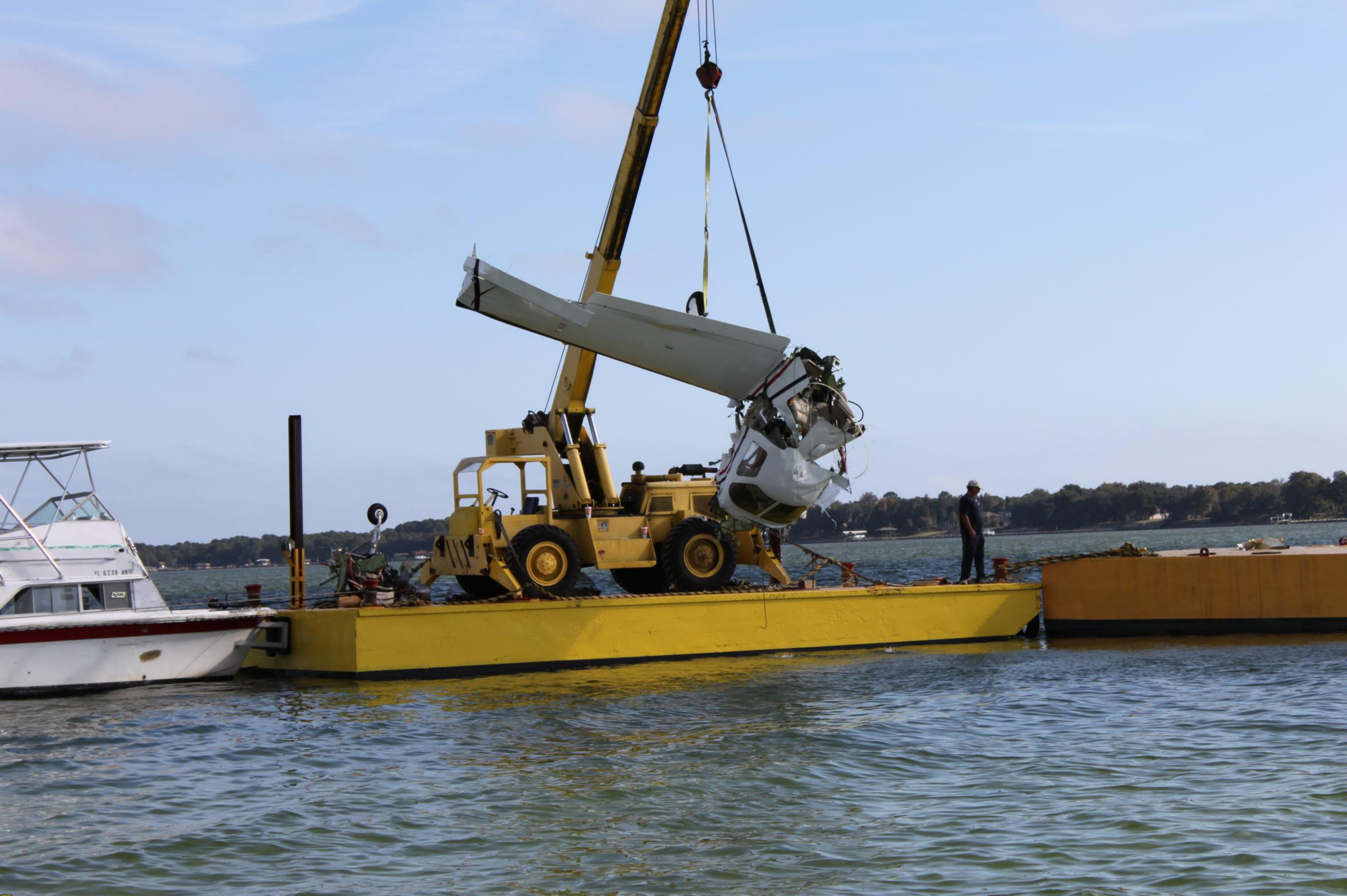
Photo 2: Fuselage and Right Wing Coming Out of the Water
