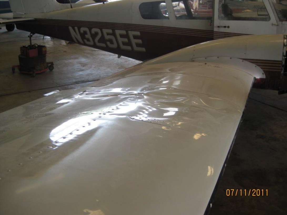
Photo 1: Digital Photograph Provided by FAA. View Showing the Damage to Right Wing.
