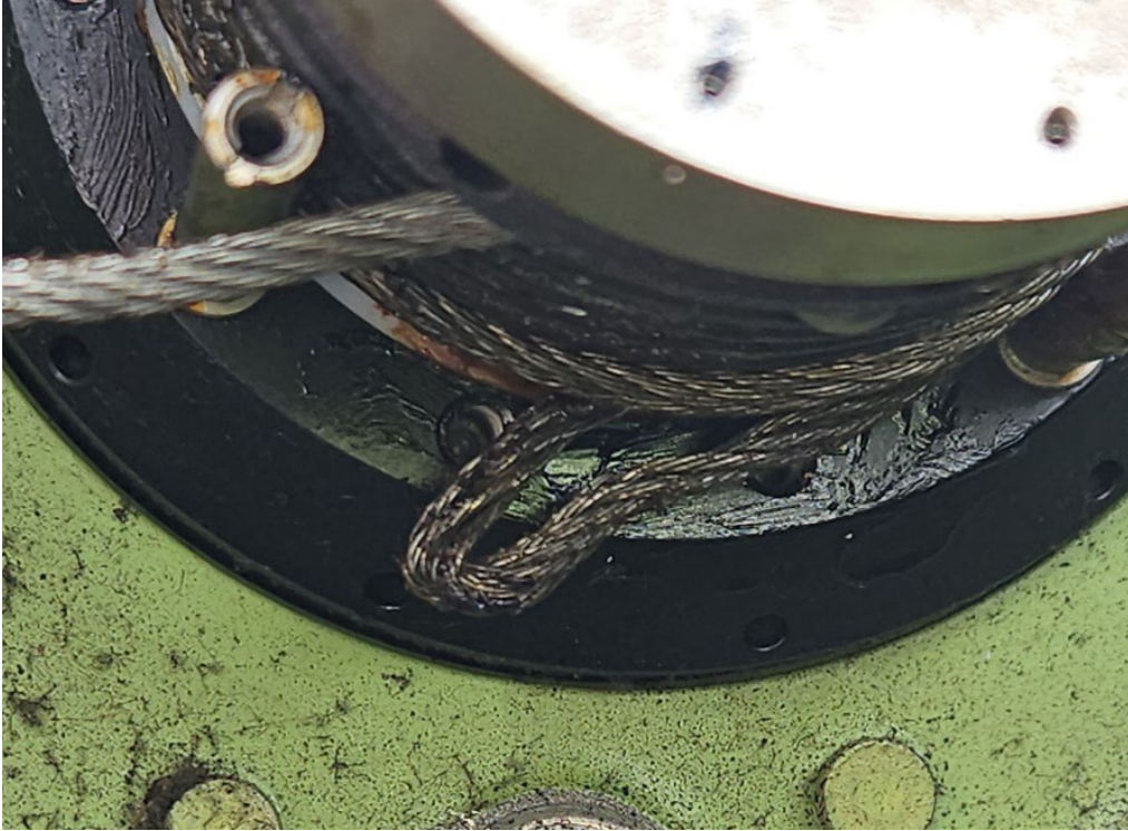
Figure 5. Cables backlashed in the elevator autopilot servo mount from the N506GJ reported event. (Courtesy of GoJet Airlines)
