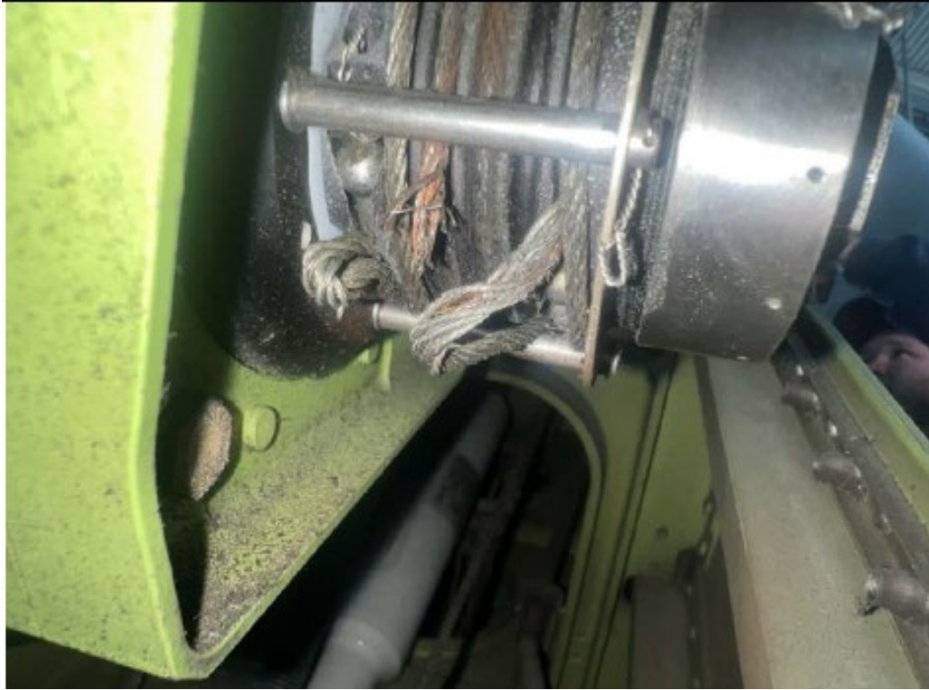
Figure 4. Cable backlashed in elevator autopilot servo mount from the N502GJ event. (Courtesy of GoJet Airlines)
