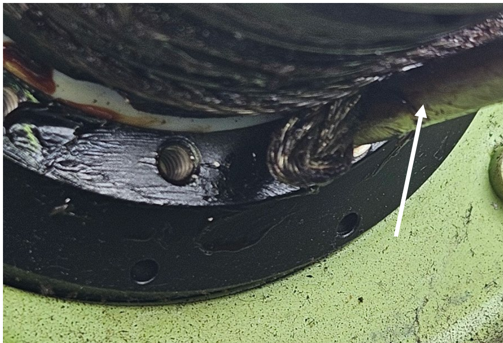
Figure 6. Cables backlashed in the elevator autopilot servo mount from the N506GJ reported event. The arrow points to a cable guide pin. (Courtesy of GoJet Airlines)
