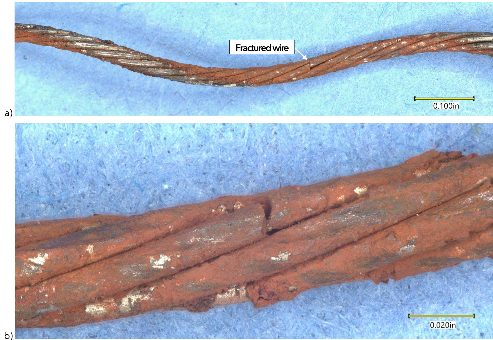
Figure 11. a) Lower magnification image of helical strand with fractured wire and b) higher magnification image of fractured wire on a second helical strand.
