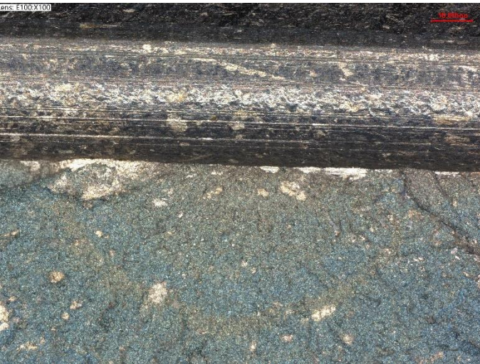
Figure 37: The OD rabbet undercut region with beach marks was examined in the SEM and shown to be fully intergranular in the larger thumb-nail-shaped region, consistent with secondary cyclic hold-time damage.
