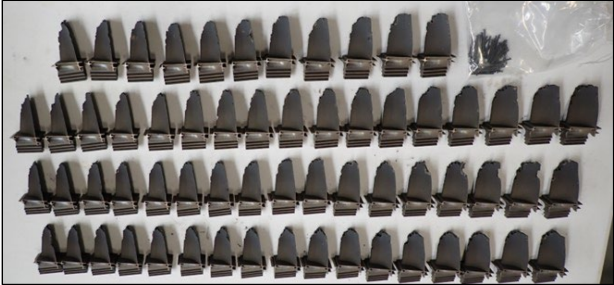
Figure 40. HPT STAGE 2 BLADE DAMAGE
