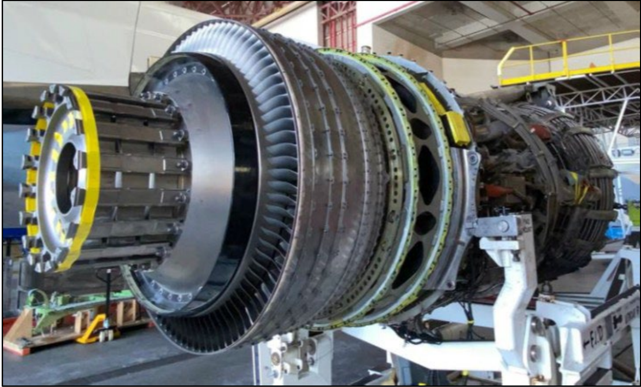
Figure 19. Engine Fan Module Removed
