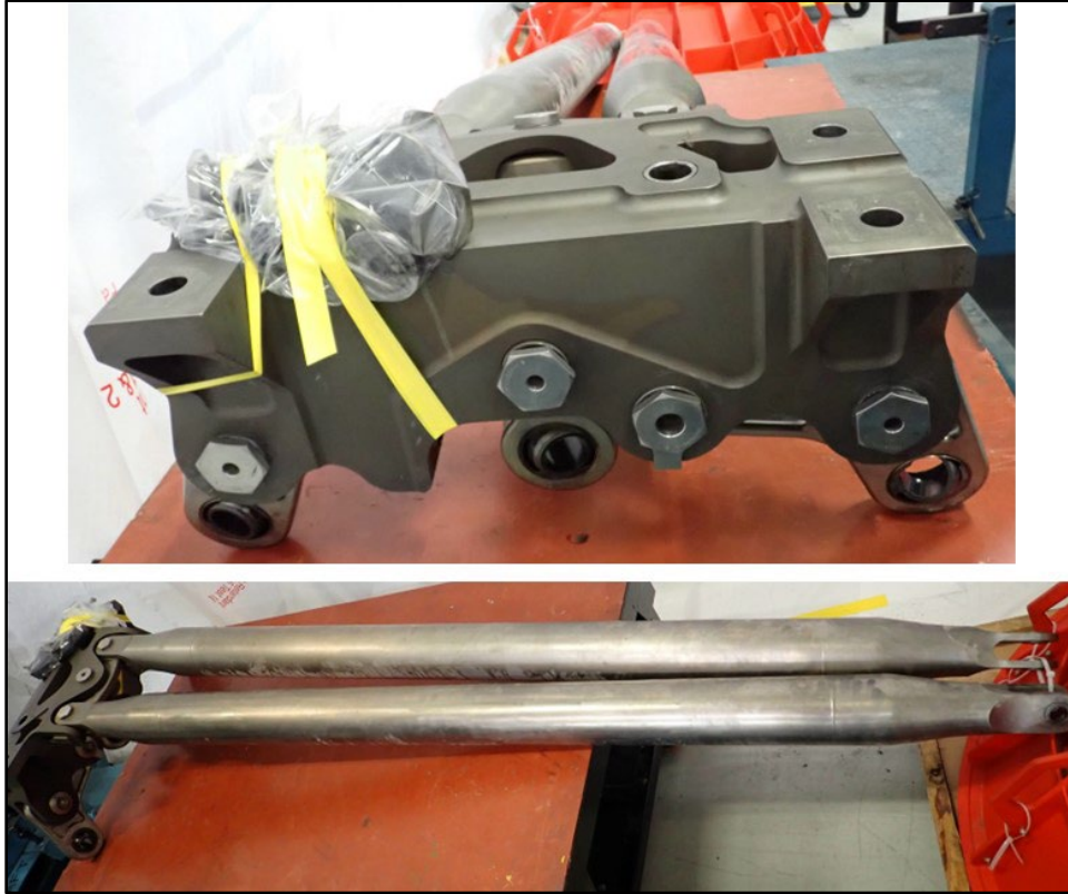
Figure 25. Thrust Links and Rear Engine Mounts
