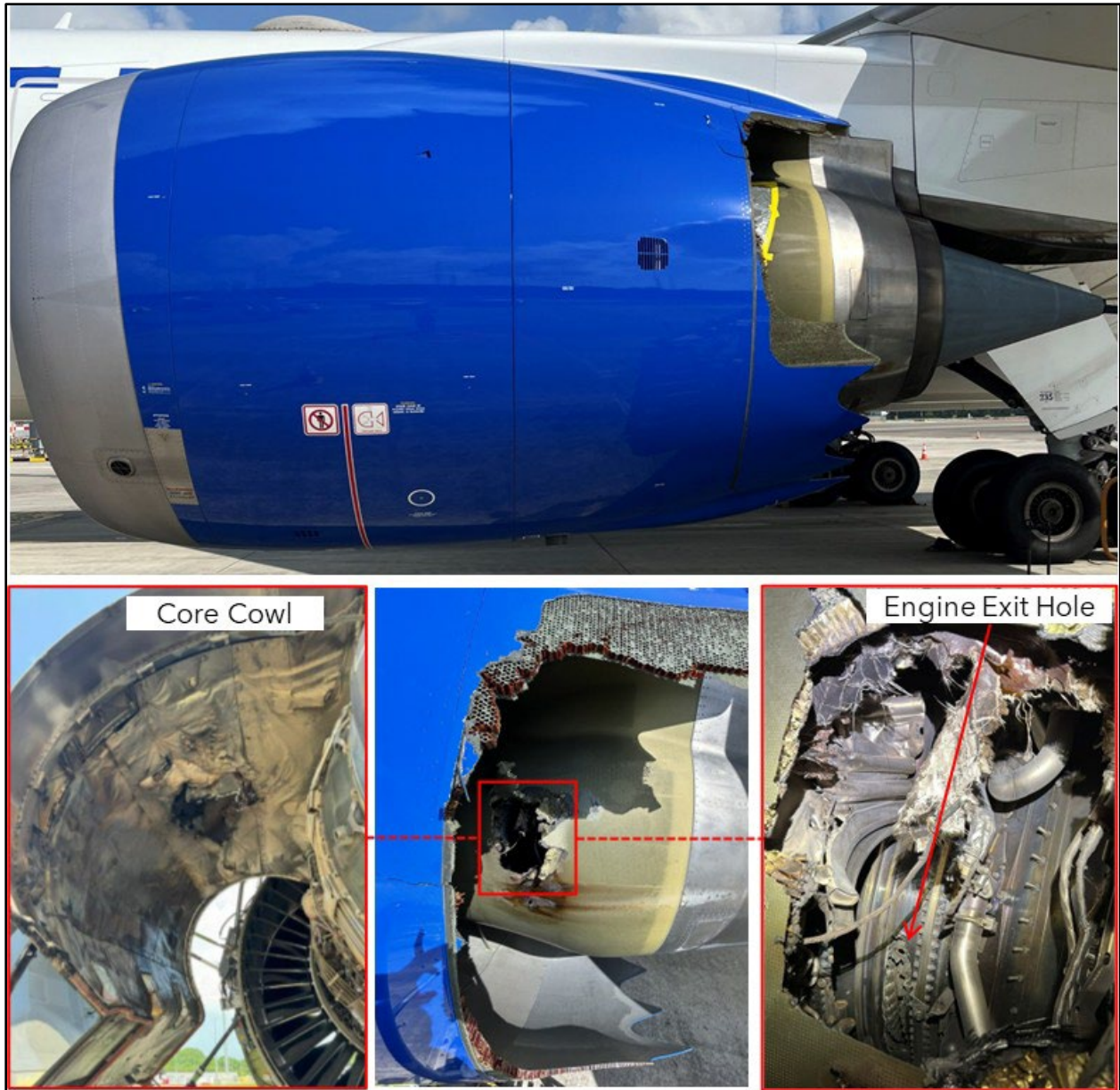
Figure 10. No. 1 Engine - Outboard Damage
