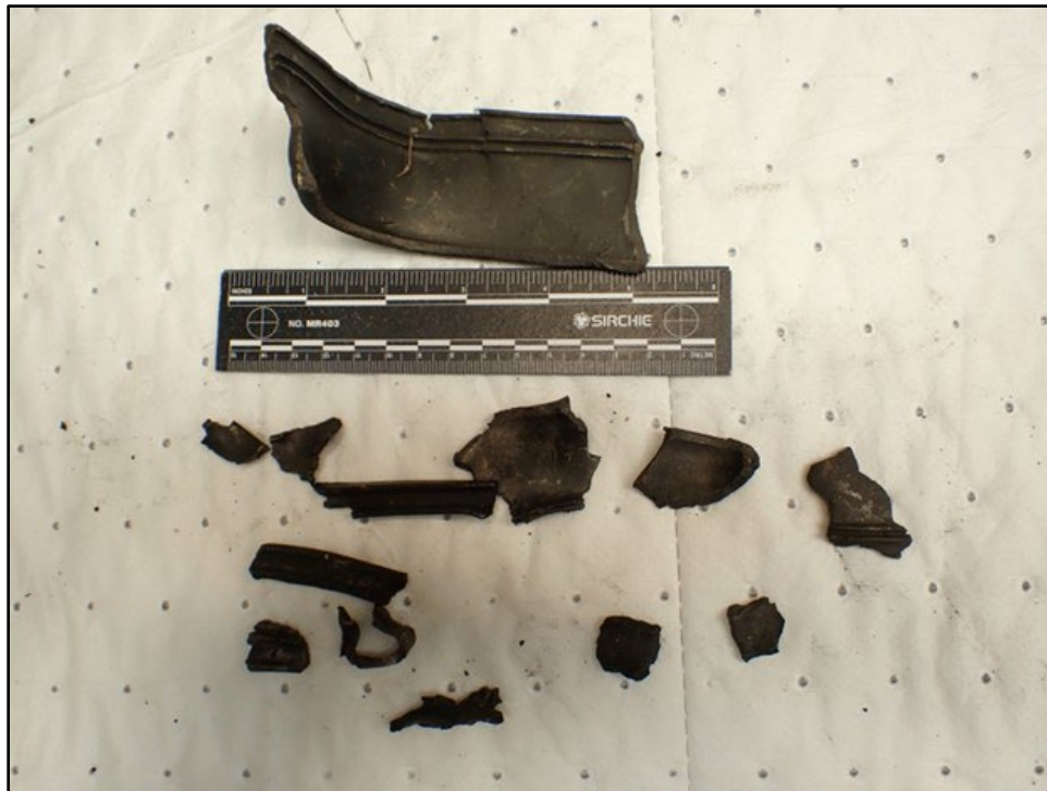
Figure 29. BOXED HARDWARE, PORTIONS OF HPT STAGE 1 AFT BLADE RETAINER
