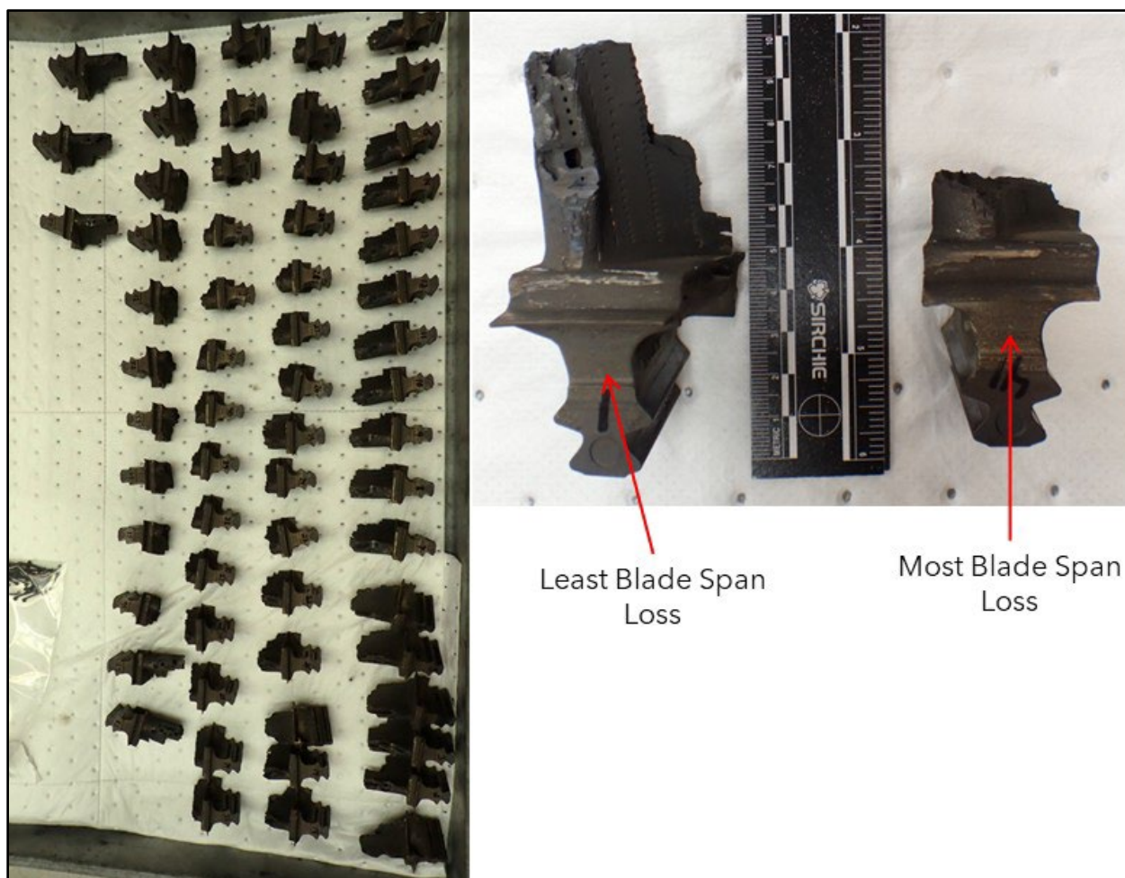
Figure 42. HPT STAGE 1 BLADES REMOVED – SHORTEST AND LONGEST
