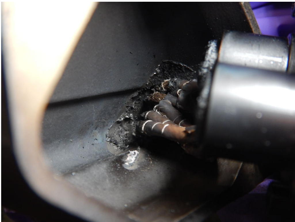
Figure 23. Resolver Wire Damage
