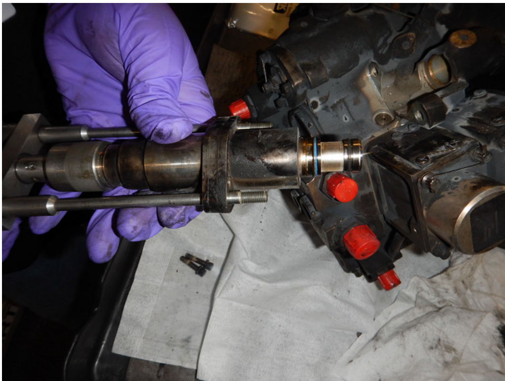
Figure 17. Airframe Shutoff Valve Solenoid
