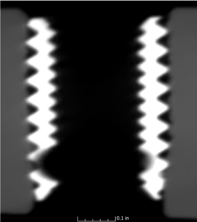
Figure 72: Optical views of insert locations 3 reveals damaged threads.
