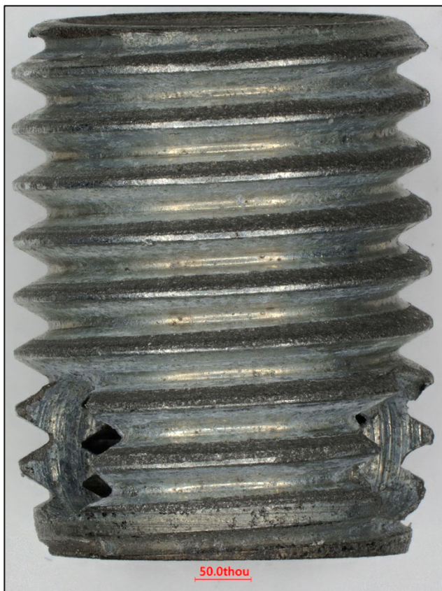
Figure 29: Images of insert 3 and 5 after removal from the flange. The major diameter of inserts 1, 3, 5, and 8 were measured and are conforming to the drawing requirement. The drilled hole diameters for holes 2 and 8 were measured at the bottom of the holes in the untapped section and both are conforming.
