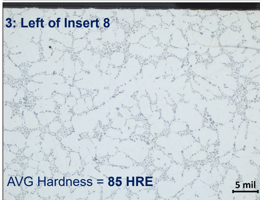
Figure 31: Cross-section images reveal a similar microstructure near holes 2 and 8. Hardness is 76 HRE near the top of the flange and increases towards the bottom, consistent with aging due to heat exposure from the fire.
