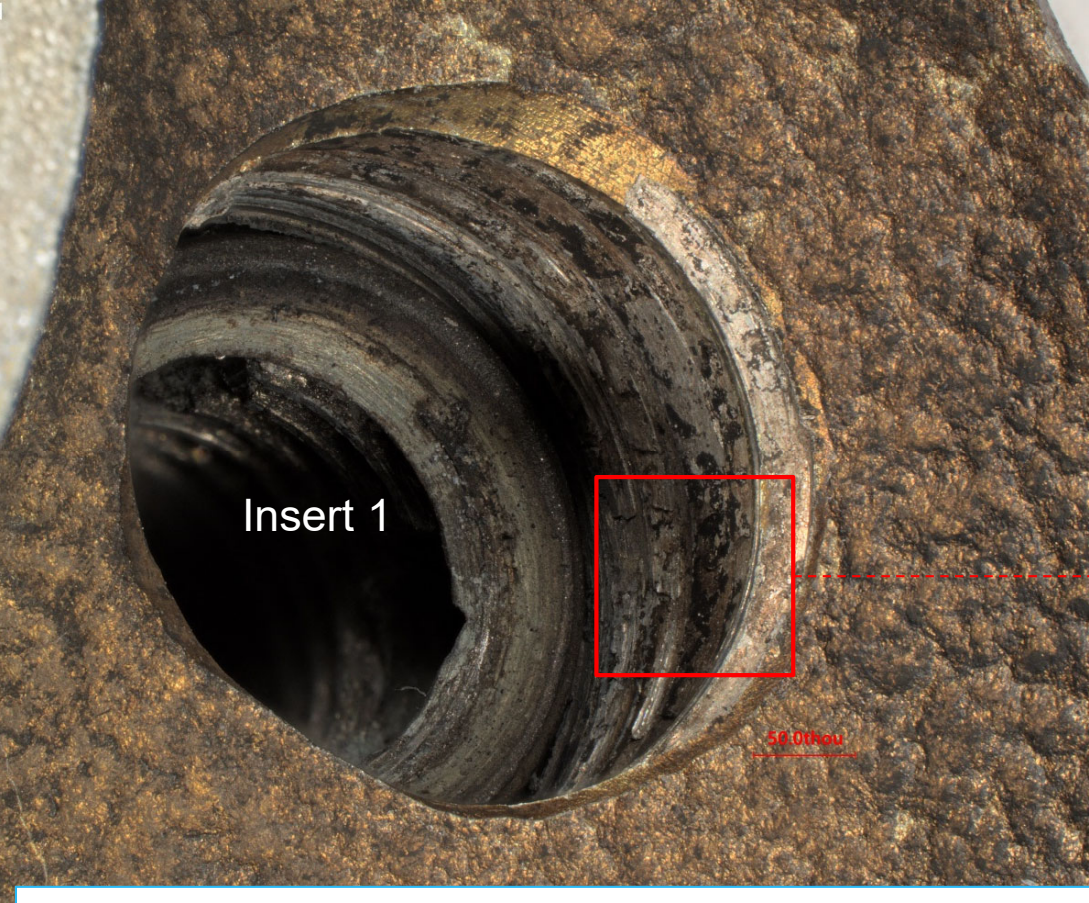
Figure 25: High magnification views of the Insert 1 hole circumferential damage reveal overlapping smear consistent with counter-clockwise rotation. Black soot-like material is observed on the smeared material, consistent with the smeared material existing during the fire.
