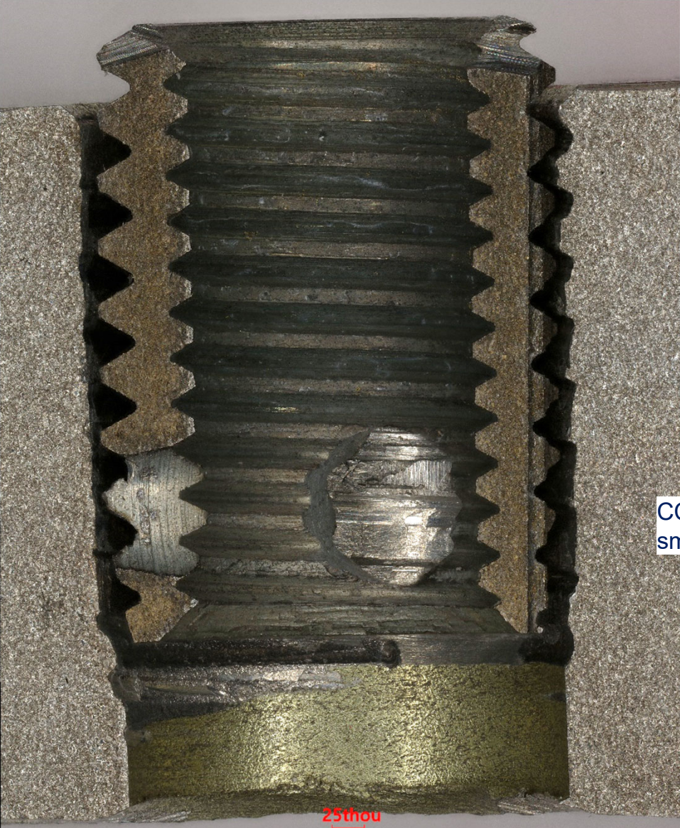
Figure 103: Optical views of insert location 8 with the inserts in place and removed. The threads are missing 360-degrees around the hole. The damaged area has vertical scoring lines consistent with the insert being pulled out. CCW smear is also observed in the damaged area.
