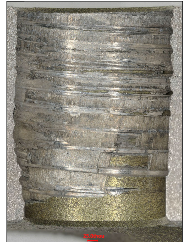
RTV FIA231MR Hole 7 (Post Pull Out Test)
