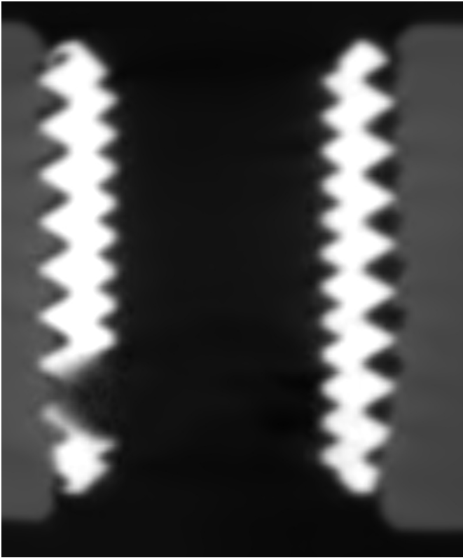
Figure 51: Optical views of insert location 3 reveals angled cut threads consistent with cross-threading. One side of the hole has a concave profile and is missing threads, while the opposite side of the hole is straight with some threads intact, consistent with the insert being installed at an angle and cutting through the pre-tapped threads.
