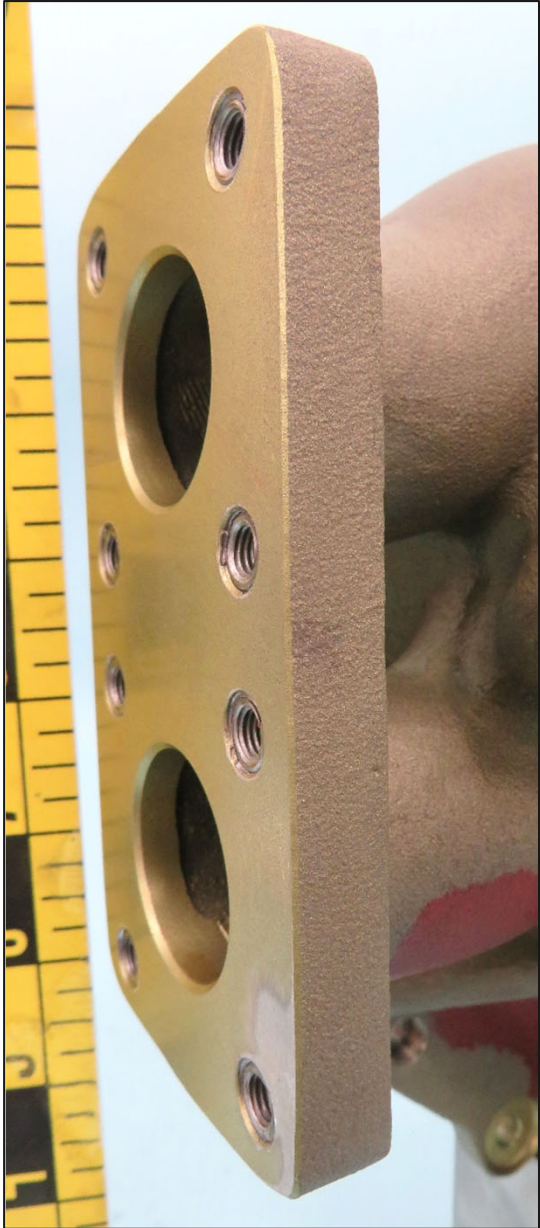
Figure 81: Images show none of the eight inserts were protruding from the flange surface. The top thread of all eight steel inserts are cracked.
